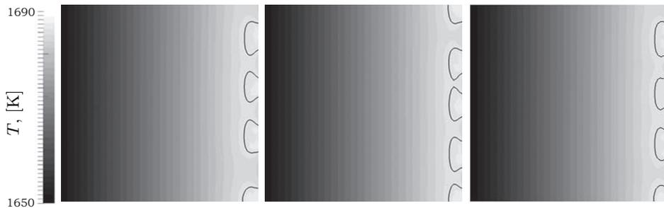
*Fig. 7.* Temperature field and phase boundaries (black lines) developed under non-uniform initial conditions (left) and with a uniform magnetic vector potential at the inductor surface. Variation of the magnetic vector potential is 2% (middle) and 4% (right).
