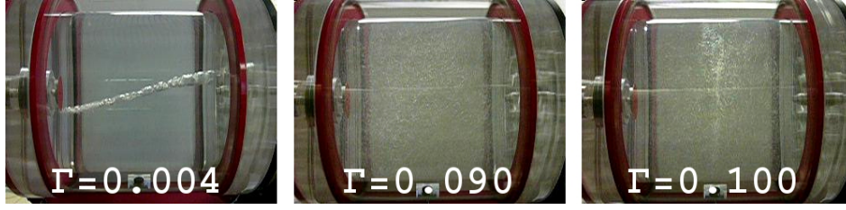
Fig. 3. Snapshots of the precessing water cylinder at different precession rates. The container axis is aligned along the horizontal plane and the system precesses around the vertical axis ( \alpha = 90^\circ ). Striking feature is the abrupt transition at the critical precession ratio \Gamma^{\text{crit}} \approx 0.07 from a laminar state (left panel) to a more disordered chaotic behavior (central panel). For even larger \Gamma the bulk fluid essentially is rotating around the precession axis (right panel).
