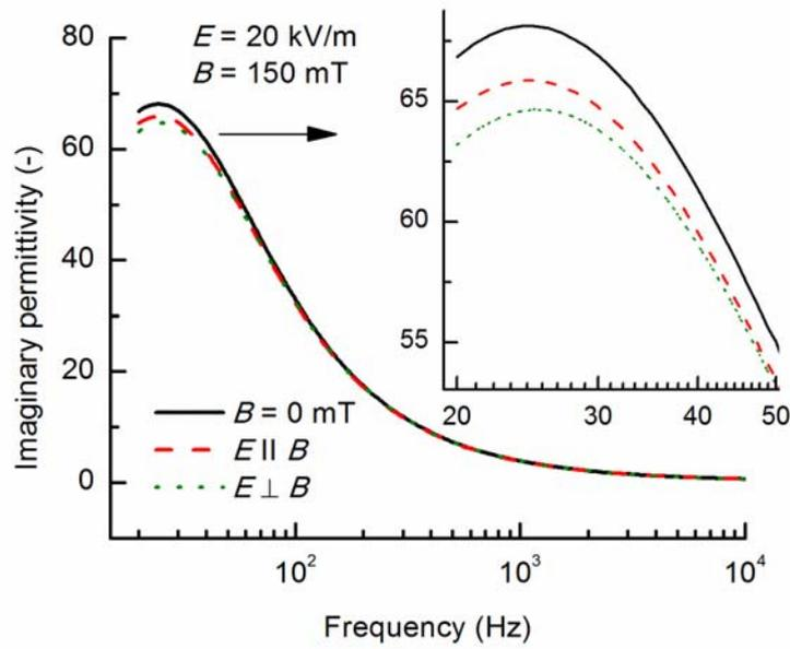
Figure 3: Magnetic field dependent imaginary permittivity spectrum.
