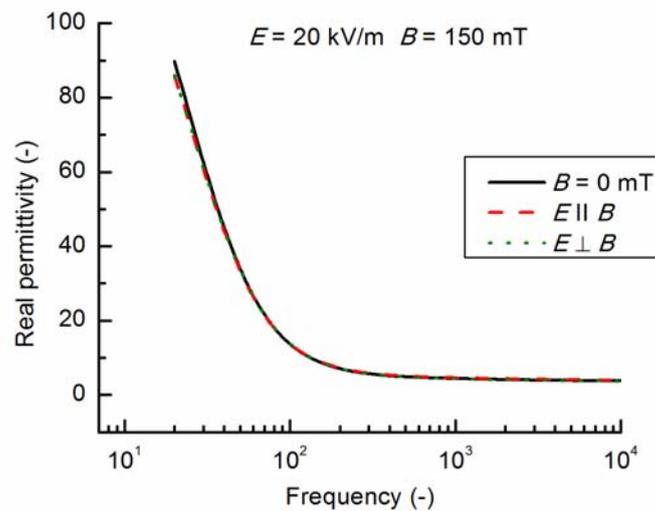
Figure 2: Influence of magnetic field on the real permittivity spectrum.
