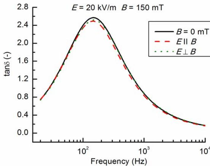
Figure 4: The influence of magnetic field on the spectrum of dissipation factor.
