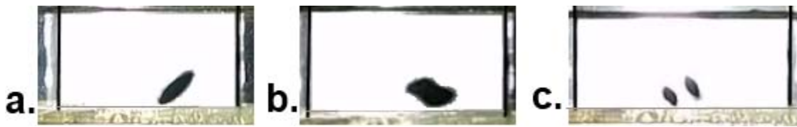
Figure 1: The MF drop shape a. H_\infty = 7.95 kA/m, \omega = 2.5 Hz; b. H_\infty = 7.95 kA/m, \omega = 5.25 Hz; c. Separation of the MF drop H_\infty = 9.94 kA/m, \omega = 4 Hz..
