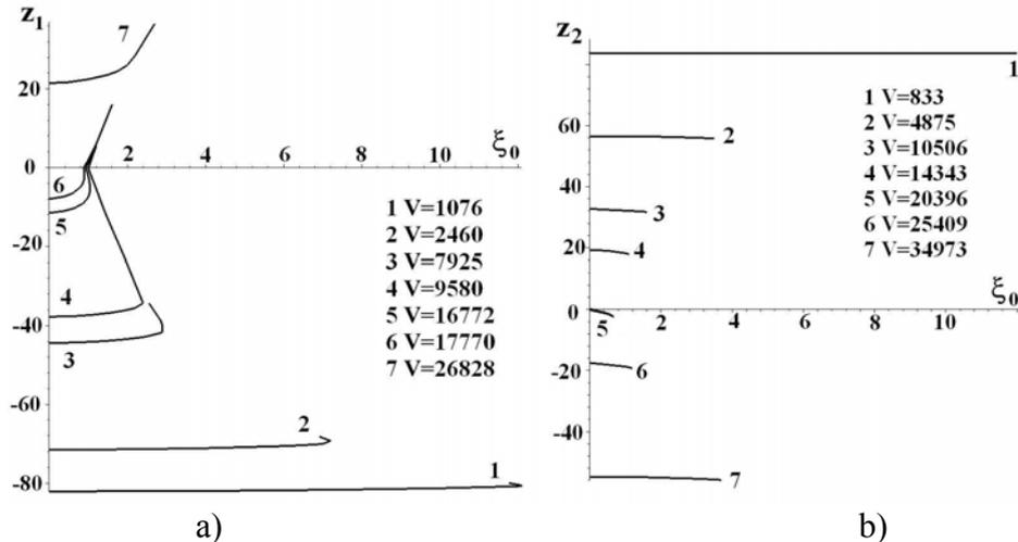
Figure 2: Dependences a)  $z_1 = z_1(\zeta_0)$  in case of non-wetting and b)  $z_2 = z_2(\zeta_0)$  in case of wetting for different values of the volume  $V$ .
