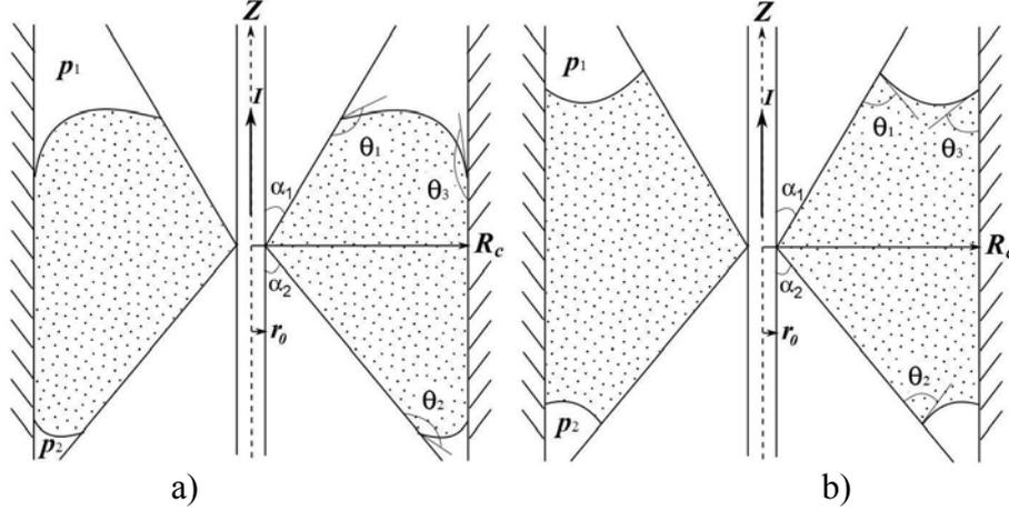
Figure 1: Ferrofluid bridge between coaxial conical and cylindrical surfaces in the magnetic field of a line conductor under a pressure drop in case of a) non-wetting and b) wetting
