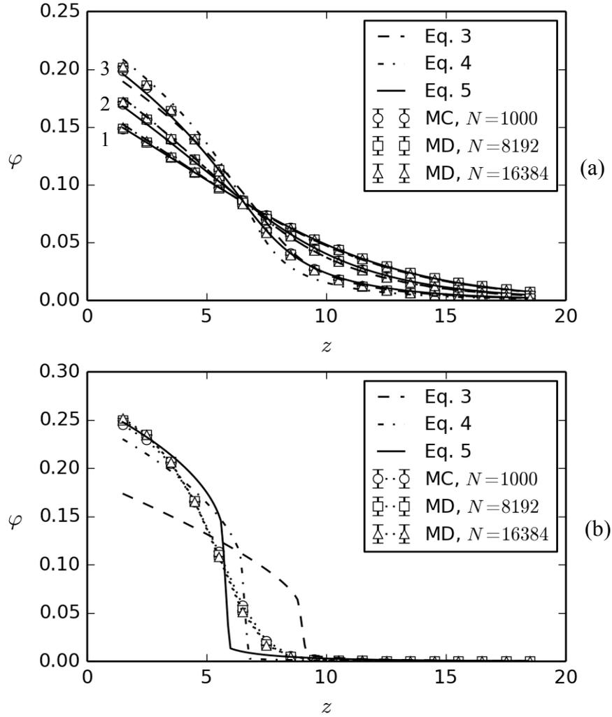
Figure 1: static concentration profiles in a vertical cylinder of finite height placed in the gravitational field. The magnetic field is absent.  $\langle \varphi \rangle = 0.06$ . Curves correspond to analytical models and markers – to numerical results. In fig. (a): curves 1 correspond to  $\lambda = 1$ , curves 2 to  $\lambda = 2$ , curves 3 to  $\lambda = 3$ . In fig. (b)  $\lambda = 5$ .
