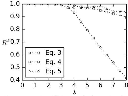
Figure 2: Coefficient of determination  $R^2$  versus  $\lambda$  for different models. The closer  $R^2$  to unity the better model approximates numerical data (MD,  $\langle \varphi \rangle = 0.06$ ,  $N = 8192$ ).
