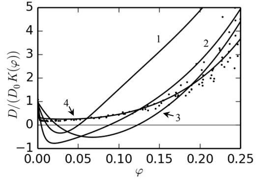
Figure 3: Diffusion coefficient versus local volume fraction for different models.  $\lambda = 5$ . Dots correspond to num. data (MC,  $N = 1000$ ), curve 1 to Eq. (3), 2 to Eq. (4), 3 to Eq. (5), 4 to Eq. (9).
