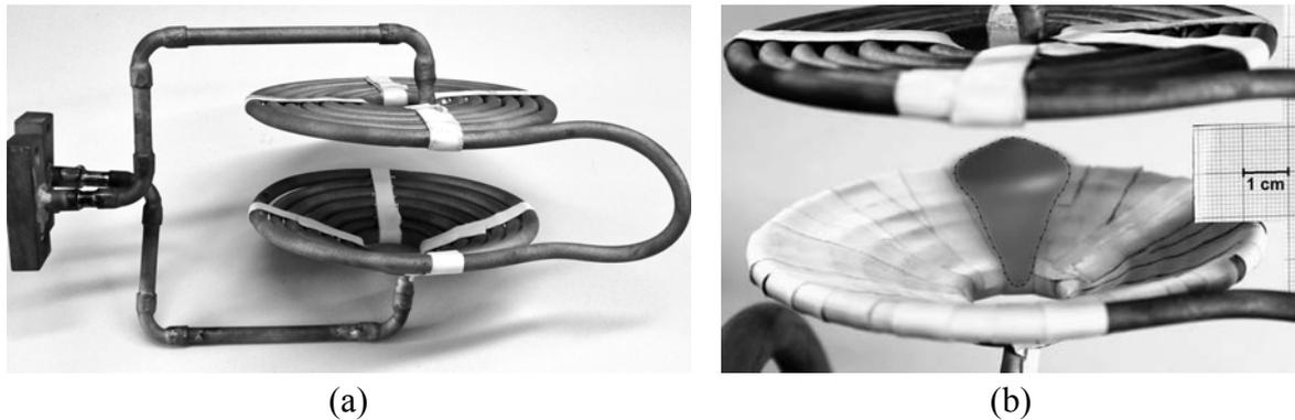
Figure 1: Our experimental setup for repeating of Okress *et. al.* levitation melting experiment (a) and a post-processed time-averaged shape of the molten aluminum sample (b).
