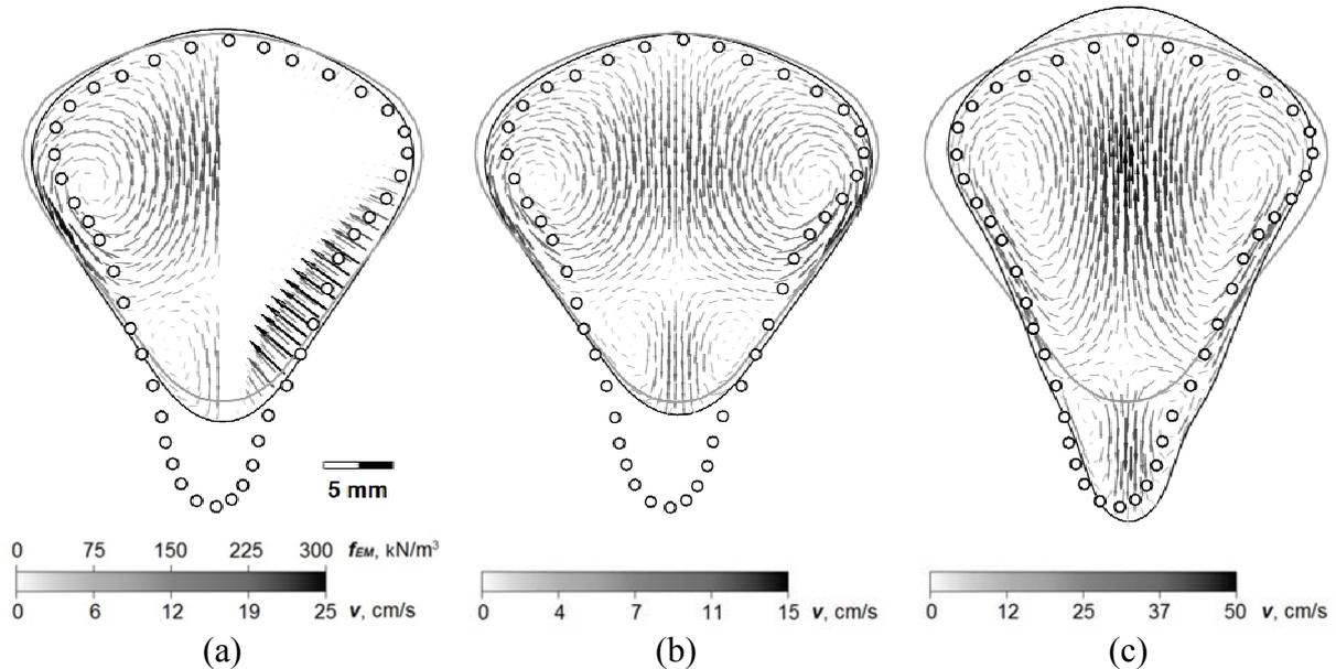
Figure 5: comparison of experimentally measured time-averaged free surface shape (O) and 2D  $k-\omega$  calculation results of V. Bojarevics (—) to our 2D  $k-\omega$  SST (a), 3D  $k-\omega$  SST (b) and 3D LES (c) time-averaged solution.
