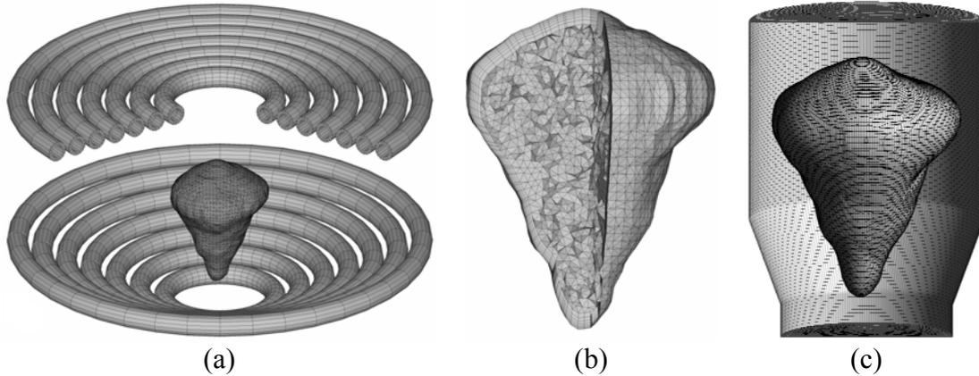
Figure 4: numerical mesh for 3D EM calculation (a) with a fine resolution of the molten metal skin-depth (b) and numerical mesh for 3D LES two-phase flow calculation (c).
