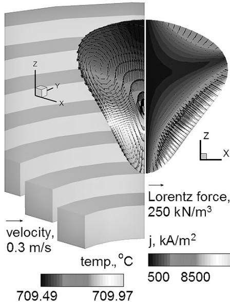
Figure 3: Velocity (on the left), EM force (on the right) and a shape of molten aluminium by V. Bojarevics *et al.* transient 2D calculation [5].
