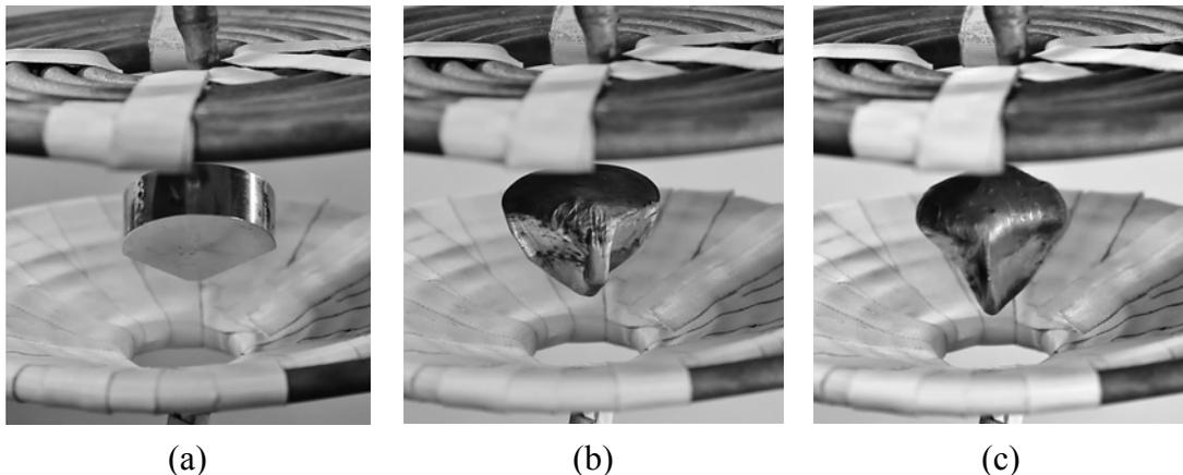
Figure 2: Solid (a), partially molten (b) and completely liquid (c) aluminium sample covered with oxide layer in our levitation melting experiment.
