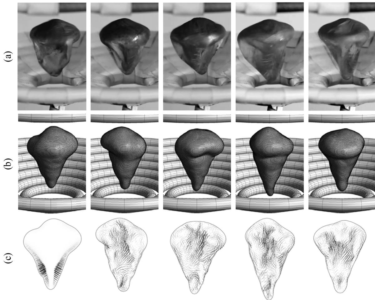
Figure 6: comparison of experimentally observed (a) and numerically simulated (b) free surface shape diversity, as well as instant EM force distribution at particular free surface shape and instant velocity patterns obtained by 3D LES simulation (c).
