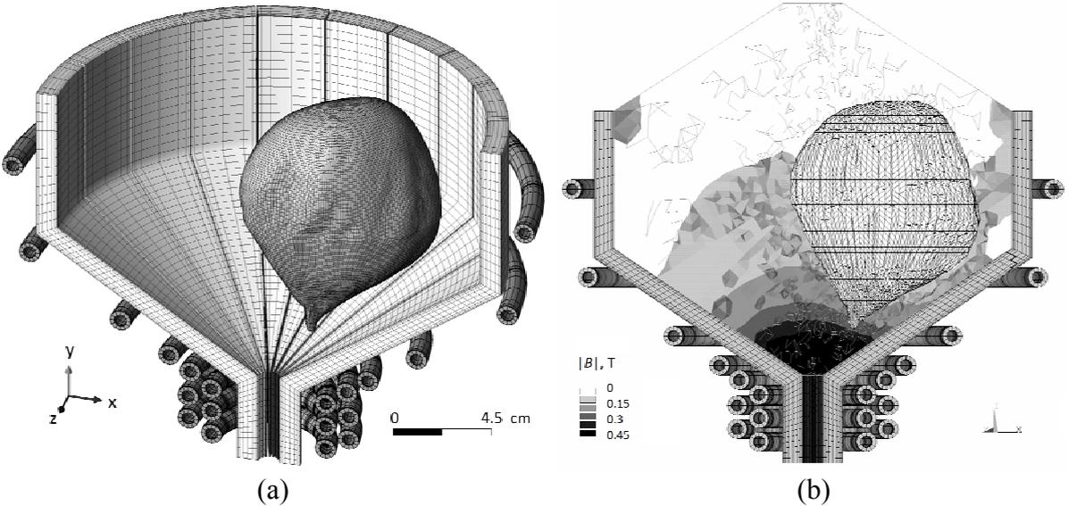
Figure 2: asymmetric position of levitated titanium (1 kg) in CC furnace with  $d_{wall} = 20$  cm obtained by 3D LES simulation (a) due to the magnetic field maximum above the nozzle (b).
