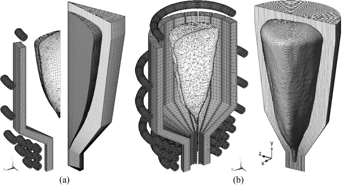
Figure 1: numerical mesh for EM and two-phase HD calculation of a molten titanium levitation. Simplified model considering a single CC section (a) and complete 3D model of CC furnace and titanium charge (b).
