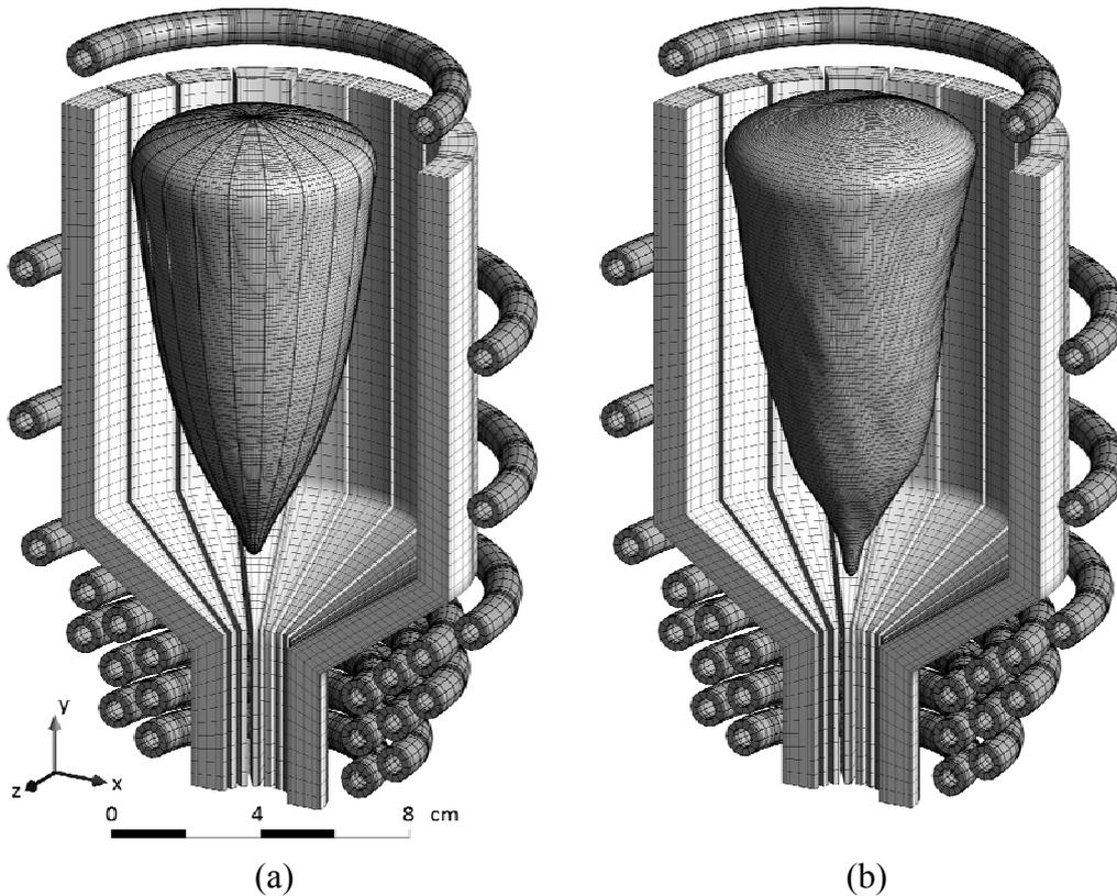
Figure 3: free surface shape of liquid titanium (1 kg) obtained by simplified  $k-\omega$  SST calculation of a single section (a) and full 3D LES simulation of CC levitation furnace (b).
