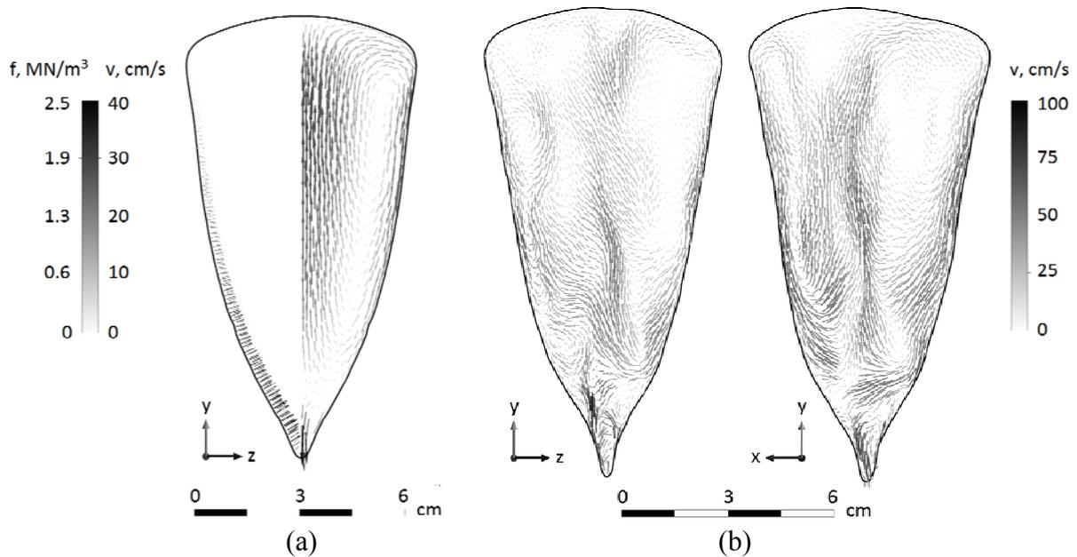
Figure 4: EM force (on the left) and flow pattern (on the right) obtained by  $k-\omega$  SST calculation of a single section (a) and instant velocity pattern calculated with full 3D LES model of CC levitation furnace (b).
