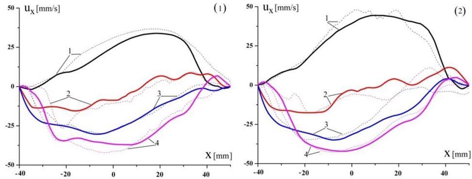
Figure 2: comparison of  $x$ -component of the flow at  $x$ - $y$  section ( $z = 20\text{mm}$ ), for different rotation velocities - 1)  $\omega_0 = 10.74\text{ rad/s}$  ( $100\text{rpm}$ ); 2)  $\omega_0 = 15.7\text{ rad/s}$  ( $150\text{rpm}$ ). Numbers on the curves correspond to  $y$ -coordinate: 1 –  $y = -23\text{mm}$ ; 2 –  $y = 0$ ; 3 –  $y = 11.5\text{mm}$ ; 4 –  $y = 23\text{mm}$ ; solid lines – computation, dashed lines – experiment (ultrasonic Doppler velocimeter DOP 2000).
