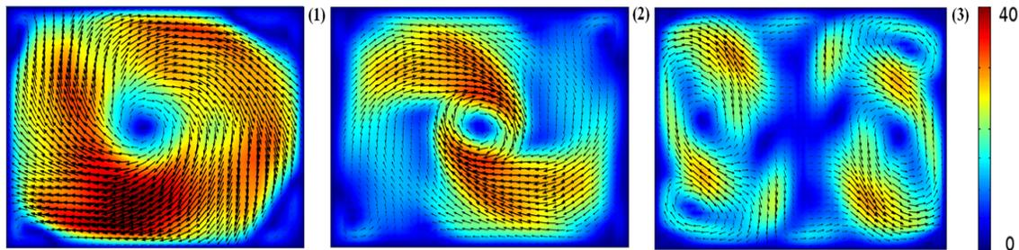
Figure 3: comparison of steady-state flow regime for different cross-sections: 1)  $x$ - $y$  plane ( $z = 20\text{mm}$ ); 2) center of  $x$ - $y$  plane ( $z = 0$ ); 3) center of  $x$ - $z$  plane ( $y = 0$ )
