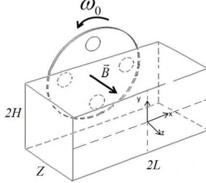
Figure 1: schematic presentation of problem statement:  $2L$ ,  $2H$ ,  $2Z$  – container's dimensions; origin of coordinates is located in the center of container (cross-section in plane  $x$ - $y$ ).
