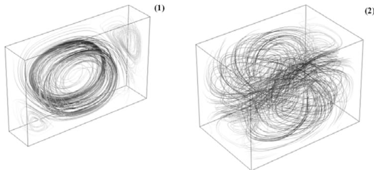
Figure 4: 3D flow patterns at  $\omega_0 = 15.7\text{ rad/s}$  in containers with different width ( $Z_{02} = 2Z_{01}$ ).
