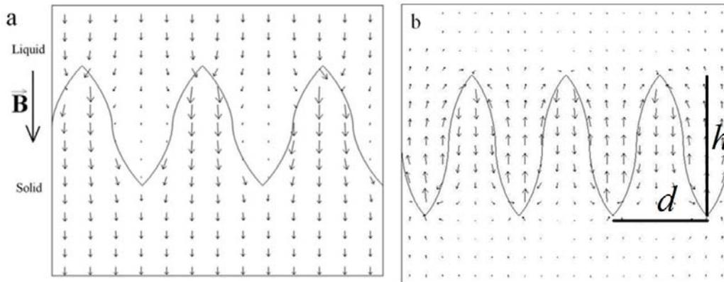
Figure 1: Conduction current redistribution at the dendritic interface due to different conductivities of solid and liquid phases: a) current distribution at the interface between two media with different conductivities; b) current component when axial current in the bulk of the liquid is subtracted.
