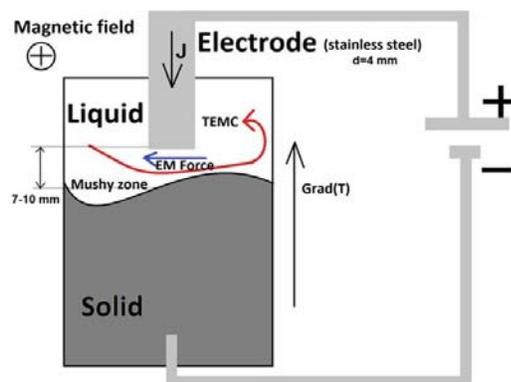
Figure 2. Experimental scheme for directional solidification with an applied electric current and magnetic field.
