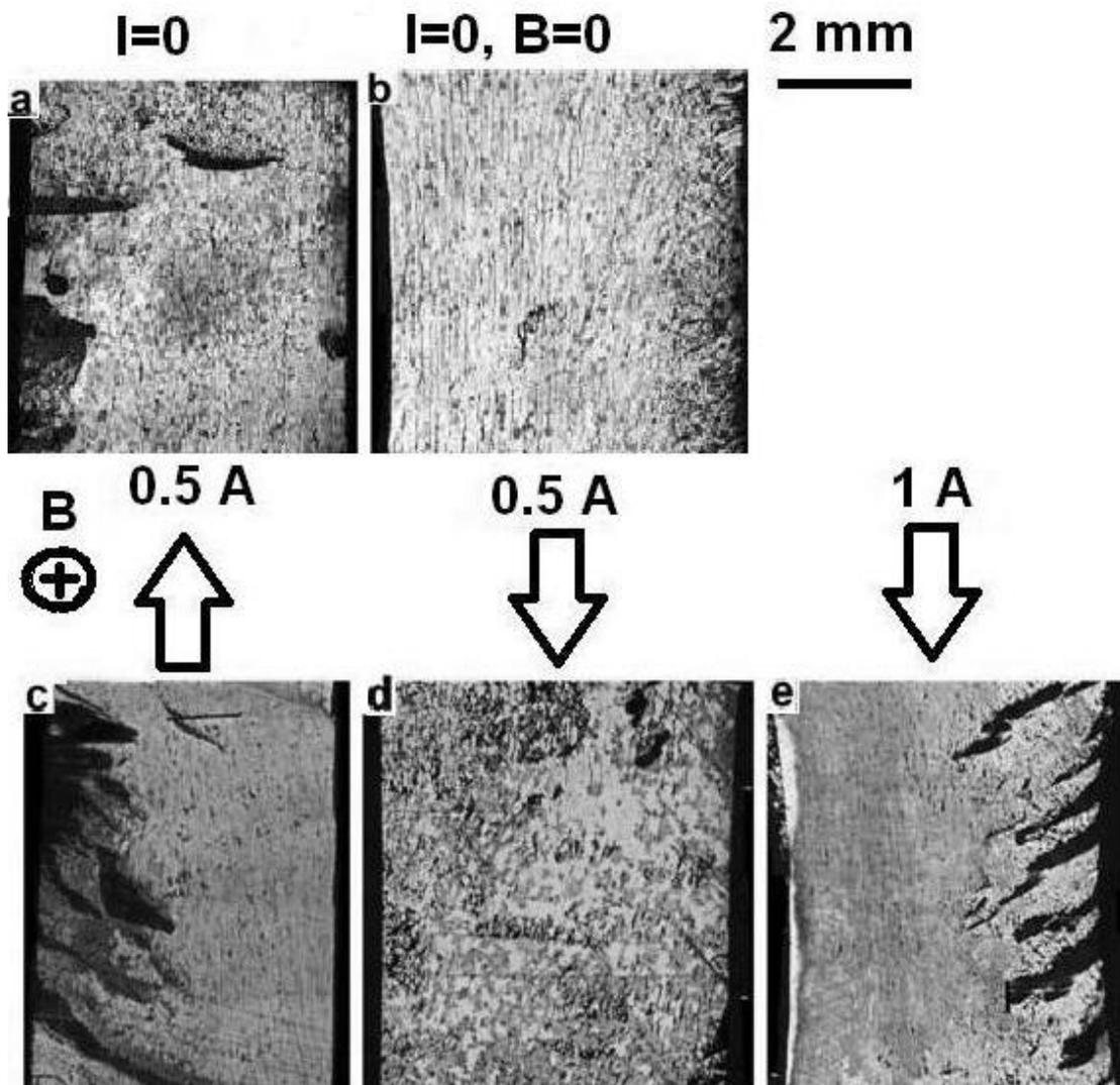
Figure 3: Directionally solidified Sn-10%wt.Pb alloy at  $v = 3 \mu\text{m/s}$  under static transverse magnetic field  $0.5 \text{ T}$  and electric current: a)  $I = 0$ ,  $B = 0.5 \text{ T}$ ; b)  $I = 0$ ,  $B = 0$ ; c)  $I = 0.5 \text{ A}$ ,  $B = 0.5 \text{ T}$ ; d)  $I = -0.5 \text{ A}$ ,  $B = 0.5 \text{ T}$ ; e)  $I = -1 \text{ A}$ ,  $B = 0.5 \text{ T}$ .
