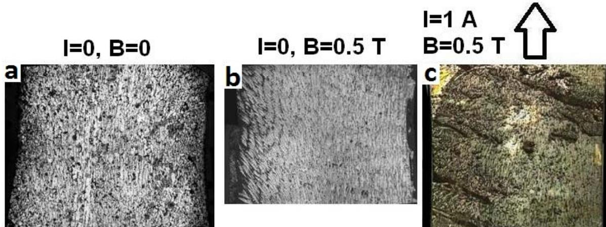
Figure 4: Directionally solidified Sn-10%wt.Pb alloy at  $v = 10 \mu\text{m/s}$  under static transverse magnetic field 0.5 T and electric current: a)  $I = 0$ ,  $B = 0$ ; b)  $I = 0$ ,  $B = 0.5 \text{ T}$ ; c)  $I = 1 \text{ A}$ ,  $B = 0.5 \text{ T}$ .
