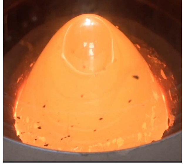
Figure 1. A schematic of the setup on the left and the semi-levitated Copper in axial 10 kHz AC field and DC field on the right.
