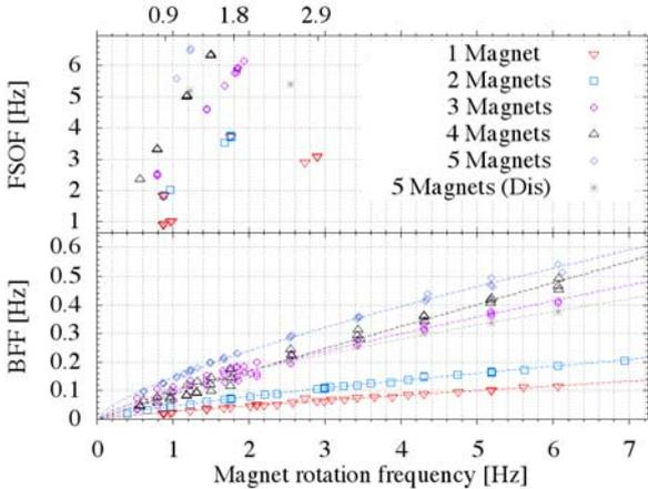
Figure 3: Bulk flow frequency (BFF) and free surface oscillation frequency (FSOF) as a function of magnet rotation frequency for all magnets arrays rotating at 42.2 mm from the axis. The notation (Dis) corresponds to the disordered array of 5 magnets.
