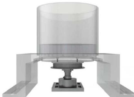
Figure 1: Sketch of the electromagnetic stirrer in cylindrical configuration.
