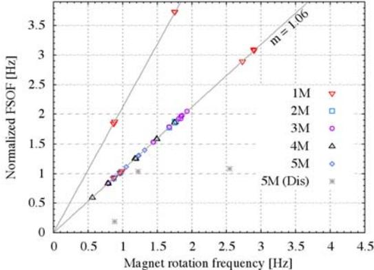
Figure 4: Normalized free surface oscillation (FSO) as function of magnet rotation frequency. Linear fitting lines correspond to  $y = mx$ , and  $y = 2mx$ , where  $m = 1.06$  is the slope of the fitted line.
