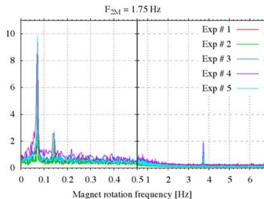
Figure 2: Maximum values of power spectra for the experiments performed with two magnets rotating at a frequency of 1.75 Hz. Note that the frequency axis was shrunk in order to show the peak at 3.8 Hz.
