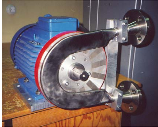
Figure 1: Photo of a typical disk-type the EM induction pump with permanent magnets (the second disk is removed).
