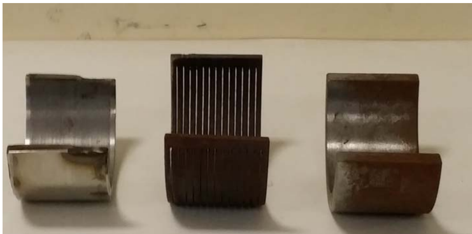
Figure 2: Different tested outer passive ferrous yokes: a) laminated; b) ferrous plate with cuts, and 3) solid ferrous yoke.
