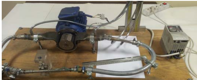
Figure 1: Experimental In-Ga-Sn loop with an EM induction cylindrical permanent magnets pump model.
