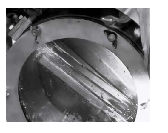
Figure 6: Two running in parallel jets. B = 4\text{T} ; V = 0.27\text{ m/s} .
