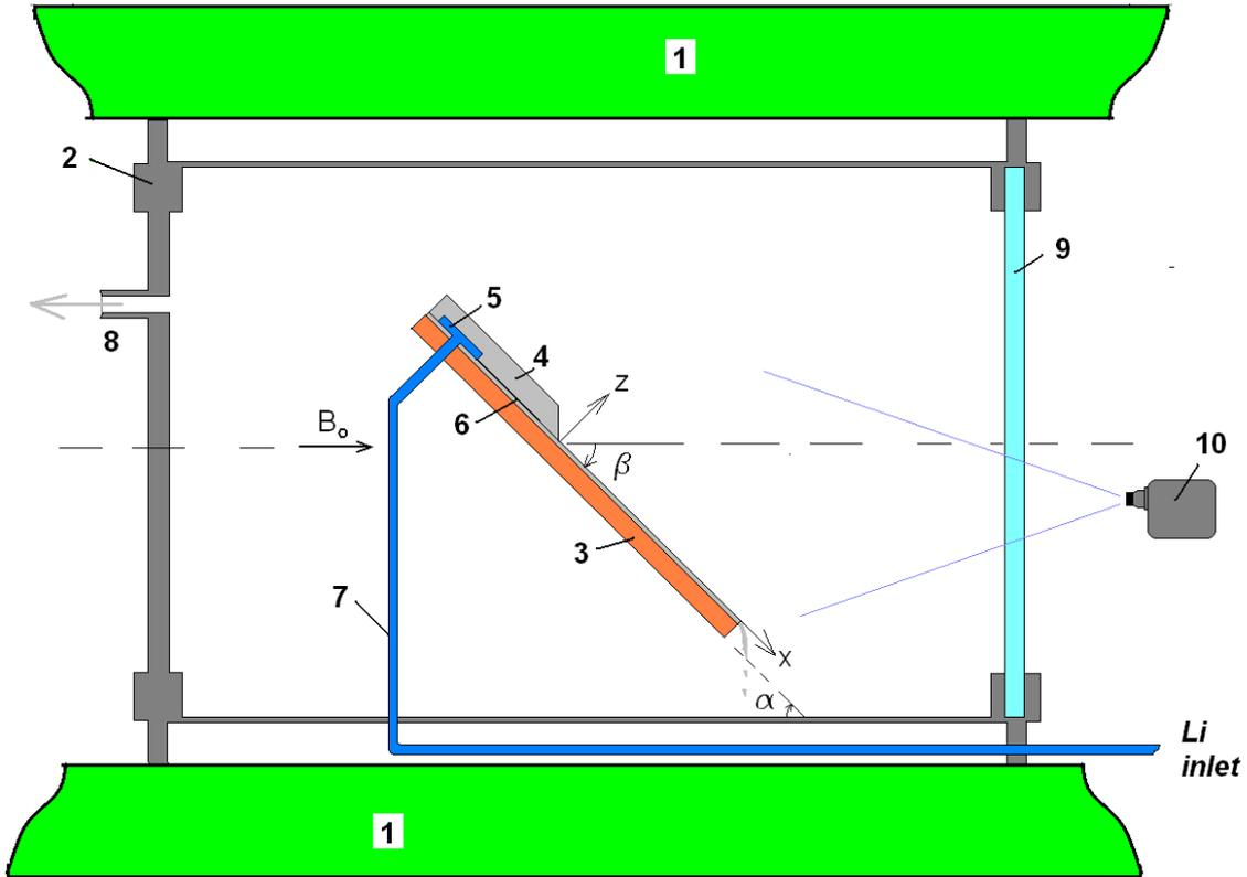
Fig.1: Schematic presentation of the experimental setup. 1 – superconducting magnet; 2 – vacuum chamber; 3 – substrate; 4 – stainless steel head; 5 – bath for liquid metal supply; 6 – zone of capillary channels; 7 – pipe for liquid metal supply; 8 – branch pipe of the vacuum system; 9 – quartz glass hole window; 10 – video camera.
