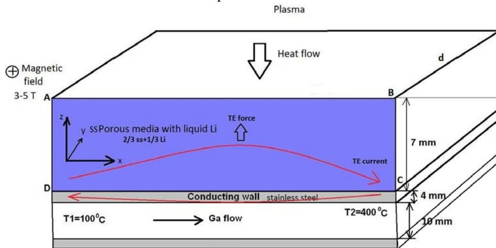
Figure 2: Schematic picture of 200x200 mm divertor plate. Thermoelectric current flow and Lorentz force are indicated with arrows.
