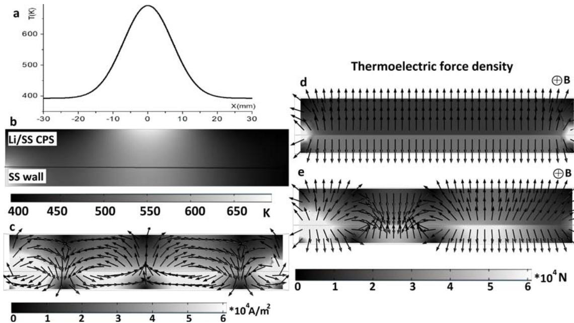
Figure 4. Thermoelectric current density if a non-homogeneous heat flux is applied. a - temperature profile along plasma/CPS surface, b - temperature distribution in the divertor plate, c - calculated thermoelectric current density. Thermoelectric force distribution in case of: d - homogeneous, e - inhomogeneous heat flow. Only CPS and SS wall are shown in this picture.
