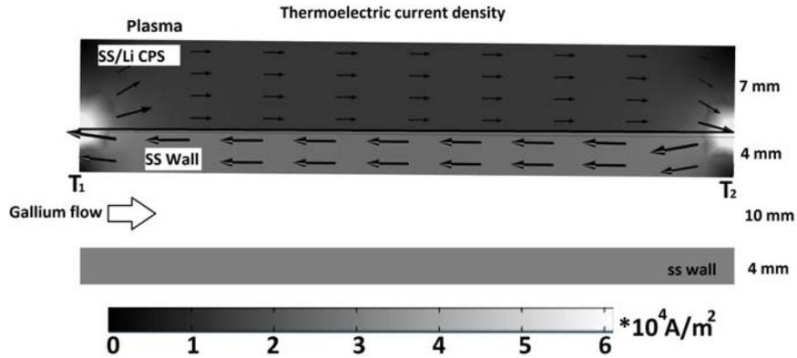
Figure 3. Thermoelectric current density in CPS region and in SS wall if constant heat flow is applied from the plasma zone.
