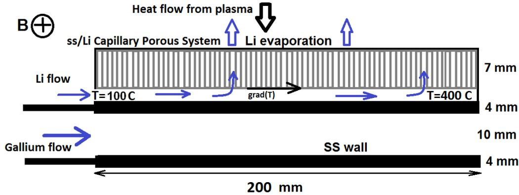
Figure 1: Li flow in the divertor. CPS here is depicted as array of the vertical stainless steel capillaries.
