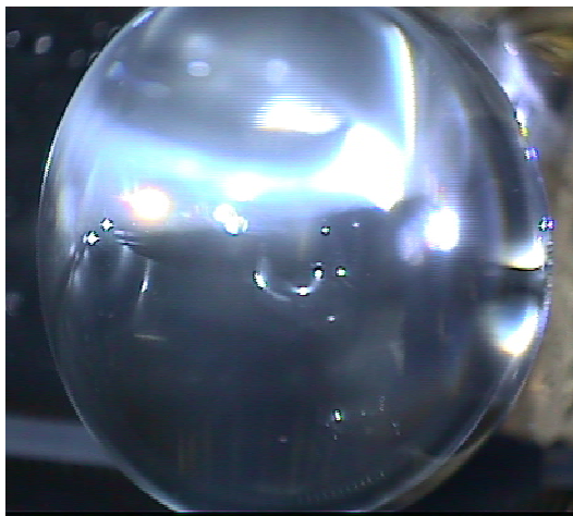
Figure 3: Images of the ethanol droplet D = 2 cm in the bore of experimental magnet and the numerically simulated (note that the vertical direction is horizontal in order to match the view from the side camera).
