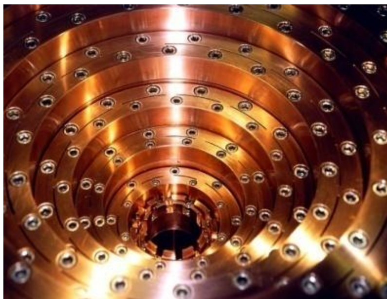
Figure: Top view of a 35 T high field magnet at LNCMI – Grenoble.
