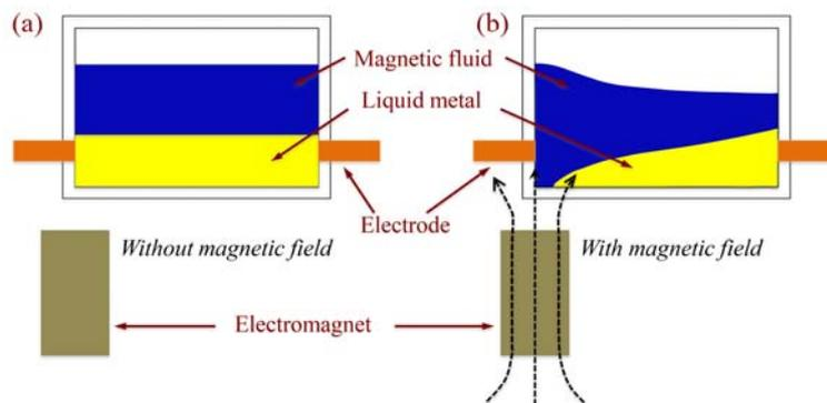
Figure 4. Principle of the binary fluids circuit breaker, (a) The state of interface when the circuit is normal, (b) The state of interface when fault current occurs.
