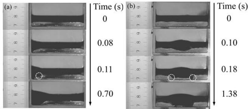
Figure 3: Interface evolution processes under weak magnetic field, (a) Side type setup, (b) Middle type setup.
