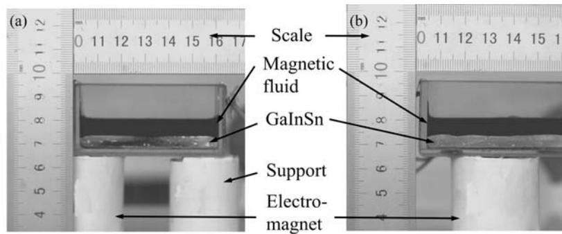
Figure 1: The experimental setups, (a) Side type setup, (b) Middle type setup.
