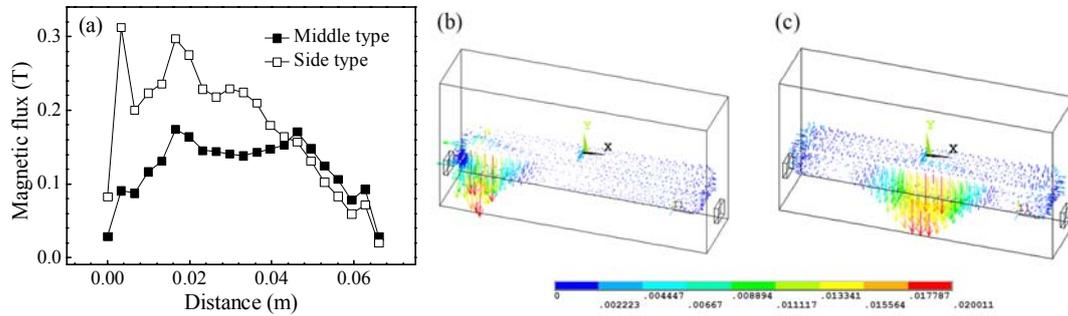
Figure 2: (a) Distributions of magnetic flux along the interface. Distributions of magnetic force, (b) Side type model, (c) Middle type model.
