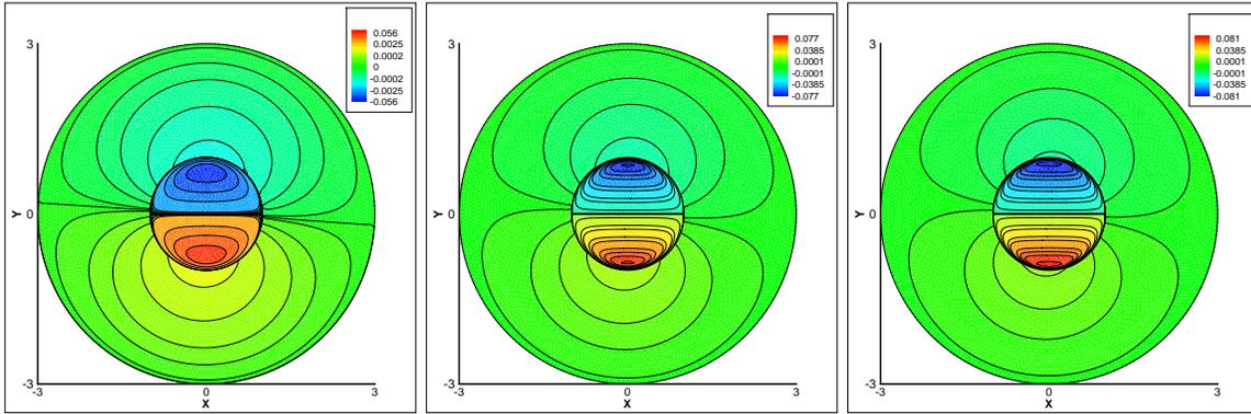
Figure 4: Induced current solution contours for  $Rm_f = 10$  (left),  $Rm_f = 50$ (center) and  $Rm_f = 100$ (right) for  $Rm_{ex} = 0.01$ ,  $Re = 1$ ,  $Rh = 10$
