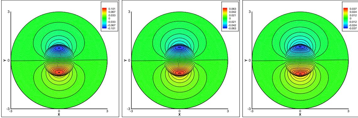
Figure 3: Induced current solution contours for  $Rh = 5$  (left),  $Rh = 10$ (center) and  $Rh = 20$ (right) for  $Re = 1$ ,  $Rm_f = 10$ ,  $Rm_{ex} = 1$
