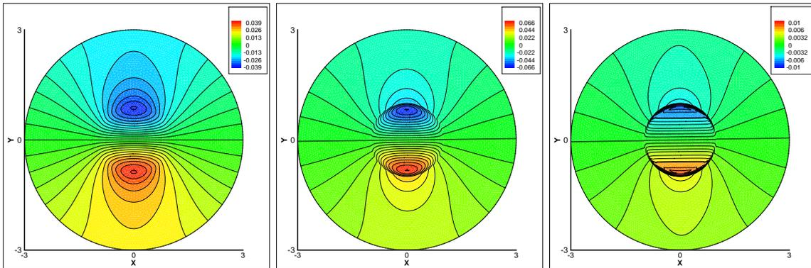
Figure 5: Induced current solution contours for  $Rm_f = 1$  (left),  $Rm_f = 10$ (center) and  $Rm_f = 100$ (right) for  $Re = 10$ ,  $Rh = 10$ ,  $Rm_{ex} = 1$
