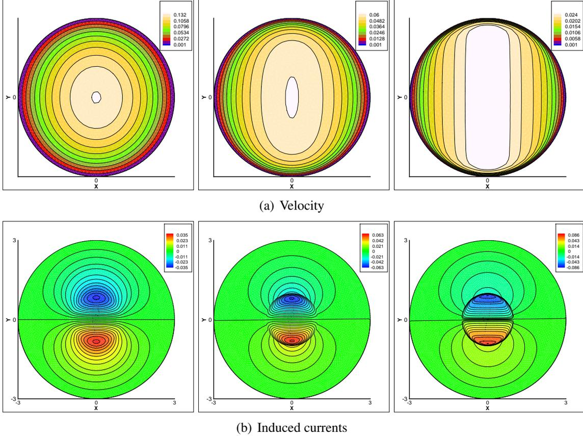
Figure 2: Solution contours for  $Rm_f = 1$  (left),  $Rm_f = 10$ (center) and  $Rm_f = 100$ (right) for  $Re = 1$ ,  $Rh = 10$ ,  $Rm_{ex} = 1$
