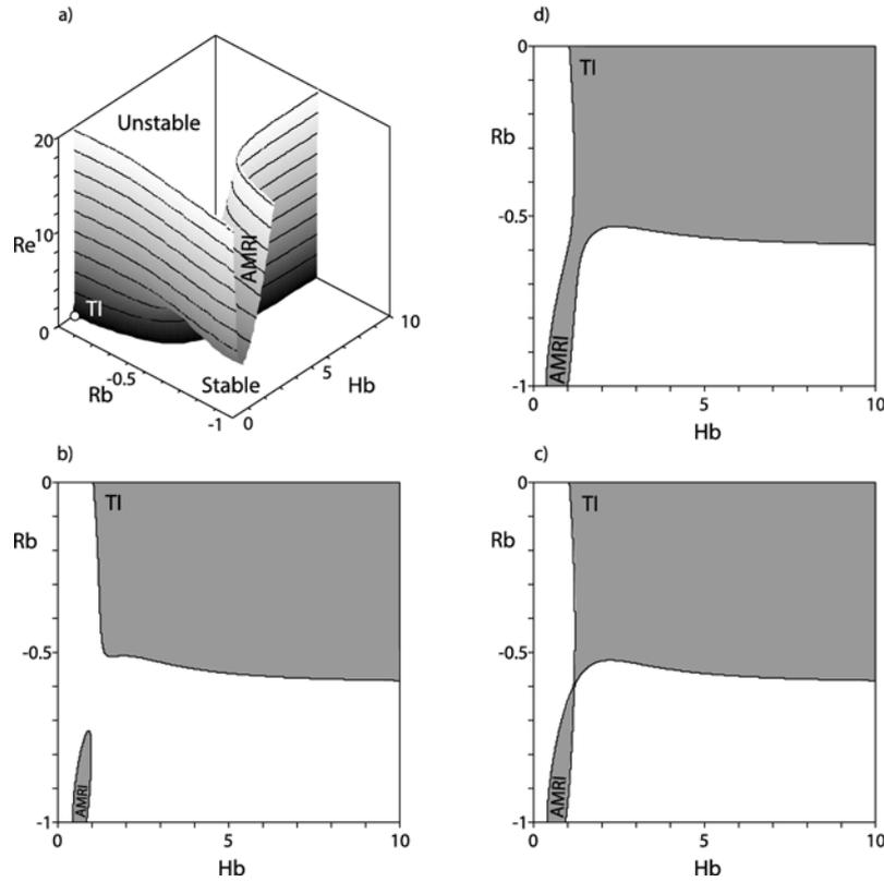
Figure 3: Instability threshold for the special case  $Pm = 0$ , and  $n \approx 1.27842$ , when following the quarter-circle curve  $Ro(Rb) = -(-Rb^2 - 2Rb)^{1/2}$ . (a) The instability domain bounded in the  $(Hb, Rb, Re)$  space and its cross-sections at (b)  $Re = 5.4$ , (c)  $Re = 5.734$ , and (d)  $Re = 6$ . The domains of TI and AMRI reconnect via a saddle point at  $Re = 5.734$ .
