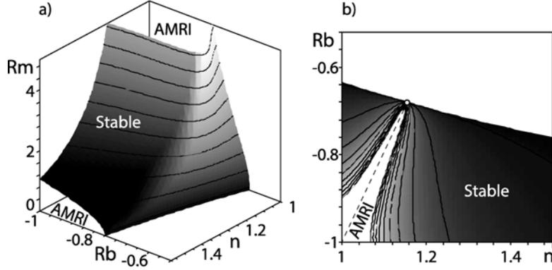
Figure 2: (a) The threshold of instability at  $Ha^2/Re = Rm$  and  $Re \rightarrow \infty$  in the  $(n, Rb, Rm)$  space. (b) Its projection onto the  $Rb$ - $n$  plane. The increase in  $Rm$  makes the instability domain more narrow so that in the limit  $Rm \rightarrow \infty$  it degenerates into a ray (dashed) that emerges from the point (open circle) with the coordinates  $n = 2/3^{1/2}$  and  $Rb = -2/3$  and passes through the point with  $n = 1$  and  $Rb = -1$ .
