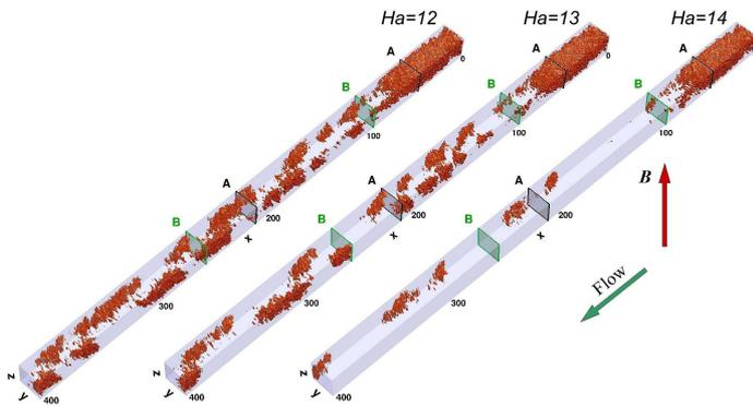
Figure 2: Patterned turbulence in spatially evolving duct flows. The isosurfaces of TKE of the transverse velocity components corresponding to 2% of the maximum are shown. Flows under stepwise magnetic field at  $Re = 3000$  are visualized for  $Ha = 12, 13$  and  $14$ . (A–A) and (B–B) indicate the pressure measurement sections, the upstream location (A) also shows the point where the magnetic field begins.
