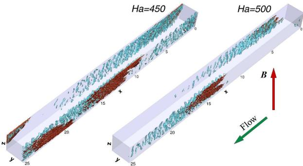
Figure 4: Patterned turbulence regimes realized in simulations of duct flow at  $Re = 10^5$  and  $Ha = 450, 500$ . The isosurfaces of TKE (brown) of transverse velocity components corresponding to 2% of the maximum are shown, also shown are the isosurfaces of the second eigenvalue  $\lambda_2$  (cyan) of tensor  $S_{ik}S_{kj} + \Omega_{ik}\Omega_{kj}$ .
