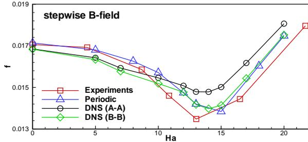
Figure 3: Friction coefficient vs. Hartmann number  $Ha$  shown for the results of simulations and experimental data (Hartmann & Lazarus, 1937).
