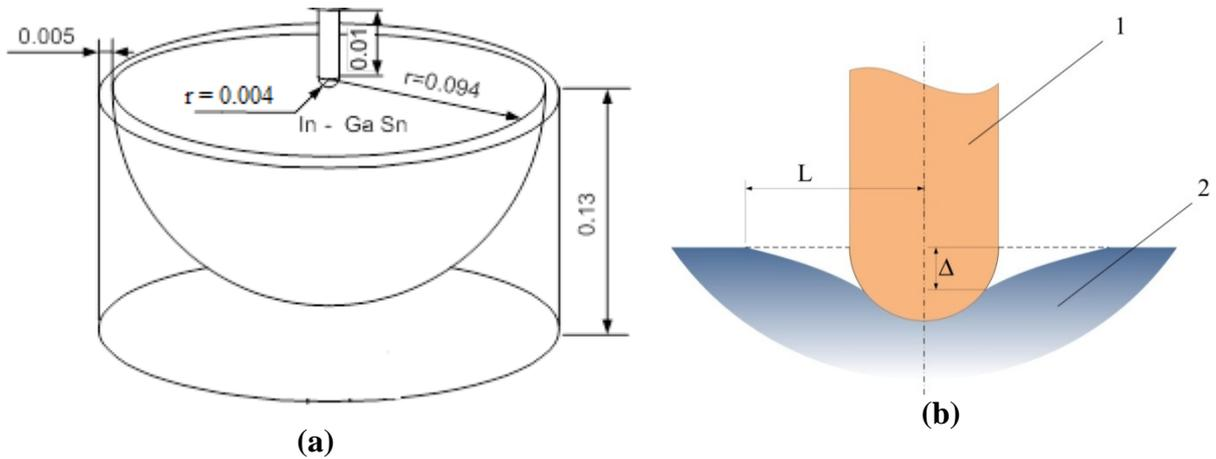
**Figure 1:** (a) dimension of the facility. (b) Scheme of surface deformation  $\Delta$  – depth of cavern,  $L$  – width of cavern, 1 –electrode, 2 – liquid metal In-Ga-Sn.
