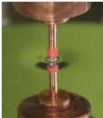
**Figure 2:** Picture of the surface of the liquid metal. A plastic gain of pink colour surrounds the tip of the electrode. A dark area near the electrode appear when the cavern becomes deep and wide enough.
