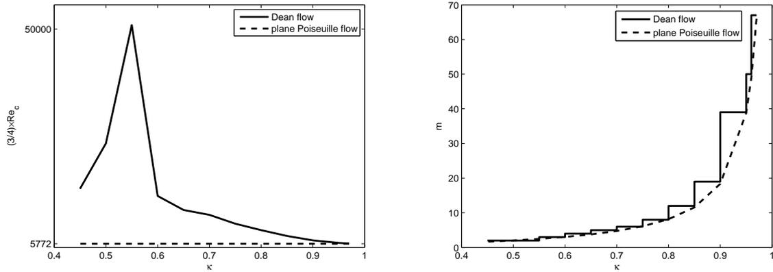
Figure 2: Stability limits of Orr modes (left) and corresponding azimuthal wavenumbers  $m$  (right) as function of the radius ratio  $\kappa$ . In plane channel flow the Reynolds number is based on the maximum velocity and the channel half-width, hence the prefactor  $3/4$ .
