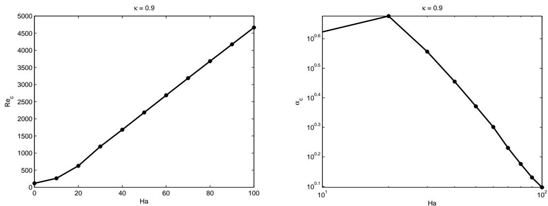
Figure 3: Critical Reynolds number of Dean mode for  $\kappa = 0.9$  (left) and corresponding axial wavenumber (right).
