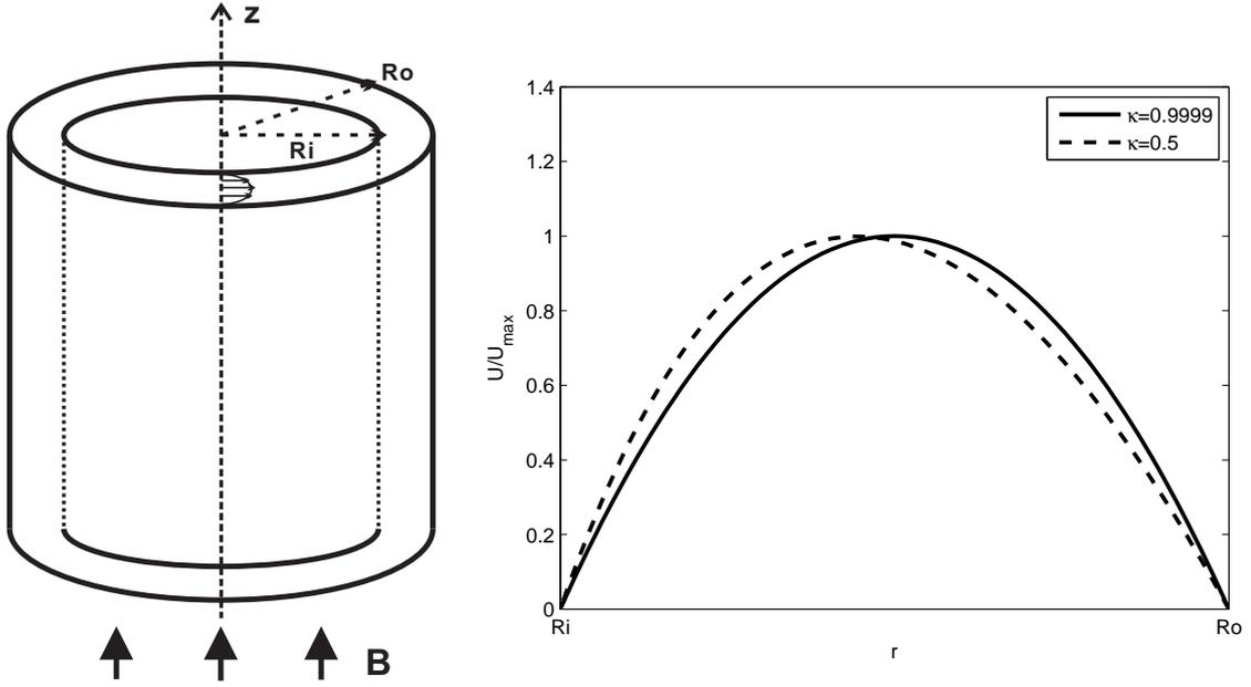
Figure 1: Sketch of the geometry (left) and basic flow structure (right)
