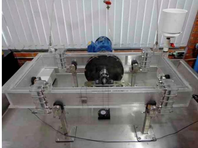
Figure 1: The experimental liquid metal loop. The MHD pump is in the far long leg. The disk and the liquid metal rotate in the counterclockwise direction. The magnet is near the middle of the near long leg, 30 cm away from the upstream corner and 4 cm over the lower wall of the duct. The ultrasonic gauge is in the far right of the picture.
