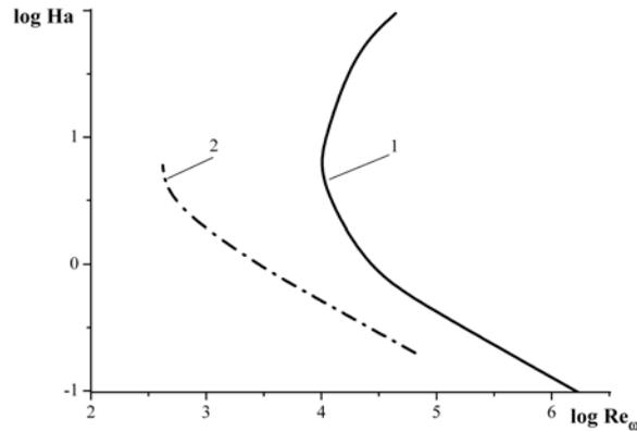
Figure 2: Estimations of neutral stability parameters for MHD flows: 1 – in helical channel, 2 – in cylindrical cavity [4].
