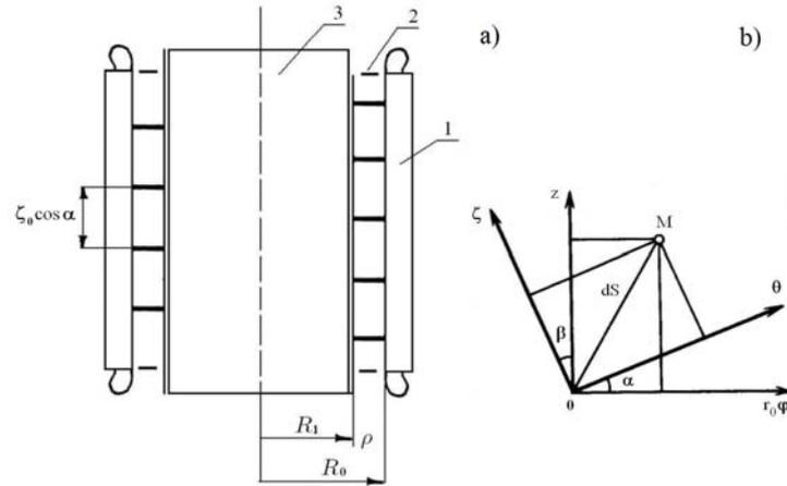
Figure1: Schematic diagram for estimations (a):1- RMF inductor; 2 - helical channel; 3 - ferromagnetic core; (b) – relations between helical and cylindrical coordinates.
