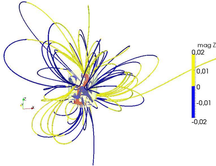
Figure 5: Snapshot at Re=1200 and Rm = 2400 of the vorticity field lines (grey/red) and the magnetic field lines colored by the axial component (light grey/yellow for positive vertical magnetic field component and black/blue for negative vertical magnetic field component).
