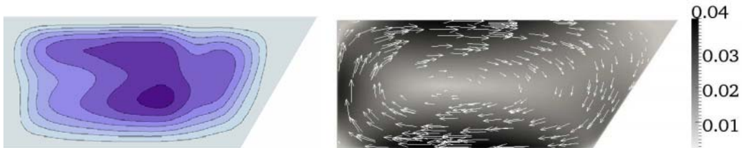
Figure 2: The flow pattern reconstructed using the experimental measurements (left) and the numerical computation results (right).
