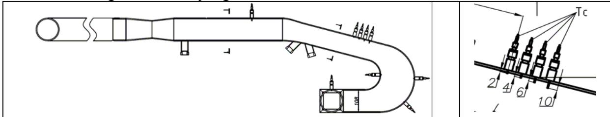
Figure 1: Test section geometry and thermocouple location.
