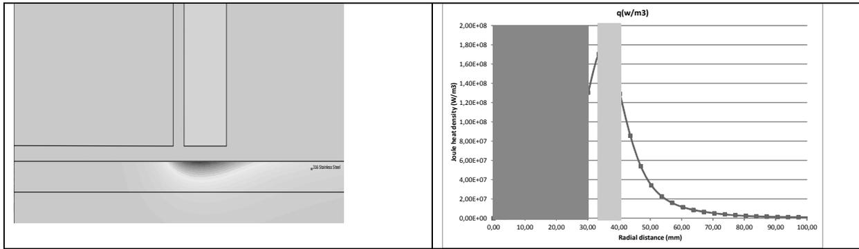
Figure 4: Magnitude of current density (left) and Joule heat source density on the wall surface (right).
