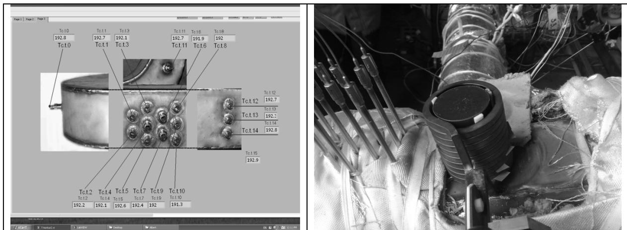
Figure 2: Thermocouple location and numbering and the inductor for heating.
