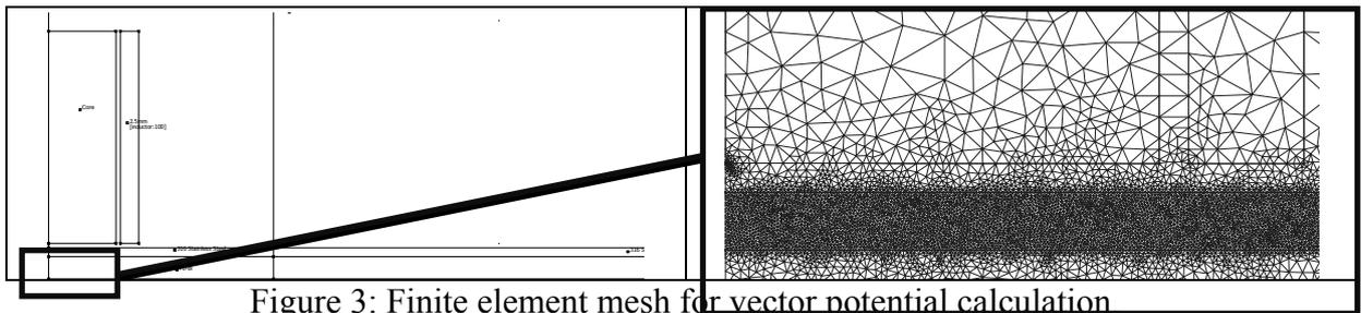
Figure 3: Finite element mesh for vector potential calculation
