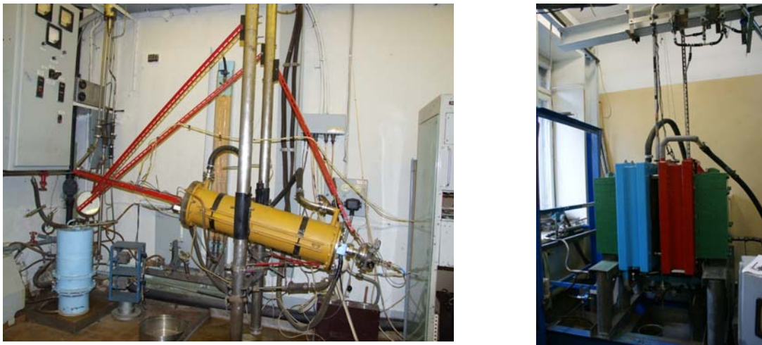
Figure 1: MPEI and JIHT RAS loop for investigations of mercury flow and heat transfer in the longitudinal and transverse magnetic field.
