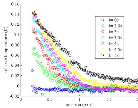
Figure 6: Temperature profile  $T(x)$  with progressing time during the magnetization phase, measured by the M-Z interferometer.
