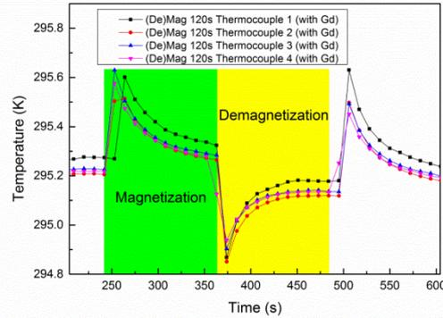
Figure 2: Temperature measurement with thermocouples during a full cycle of magnetization and demagnetization over 120 s.
