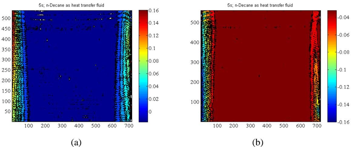
Figure 5: M-Z Interferometer measurement of temperature field in n-decane: (a) 5 s after magnetisation and (b) 5 s after demagnetisation.
