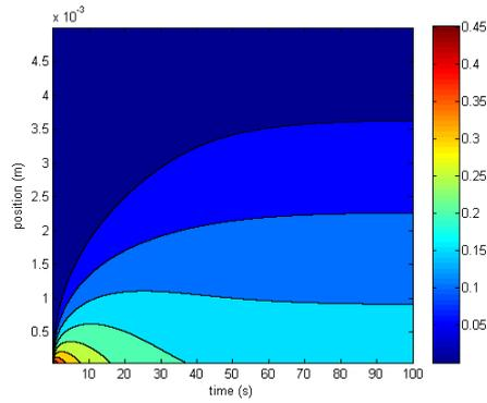
Figure 4: 1-D temperature profile versus time at the center of the Gd plate as obtained from 1-D simulation of the unsteady heat conduction equation (1) of the MCE with n-decane.
