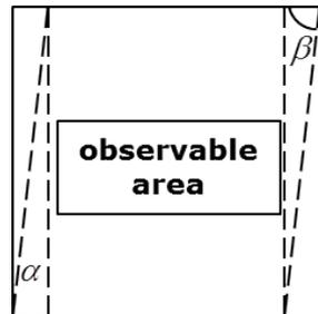
Figure 7: Sketch of the observable area of the M-Z interferometer caused by a small tilt of the Gd plates in the optical cell.
