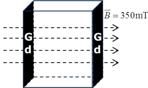
Figure 1: MCE measurement under a homogeneous magnetic field
