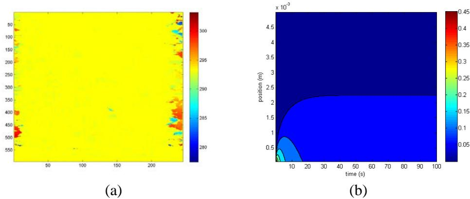
Figure 3: (a) M-Z Interferometer temperature measurement of heat transfer from 2 magneto-caloric plates into water; (b) 1-D unsteady thermo-diffusion simulation of heat transfer into water between two parallel magneto-caloric Gd plates.
