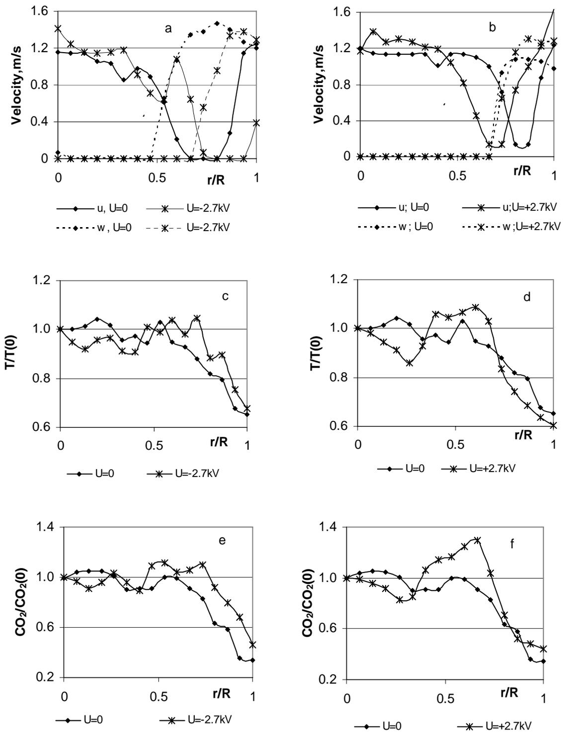
Figure 2: DC electric field effect on the formation of flame velocity (a, b), temperature (c, d) and composition (e, f) profiles at constant bias voltage ( $U = \pm 2.7$  kV) and variations of DC field polarity.
