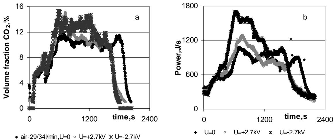
Figure 1: DC electric field effect on the kinetics of CO<sub>2</sub> formation (a) and heat power production (b) at thermo-chemical conversion of biomass pellets.
