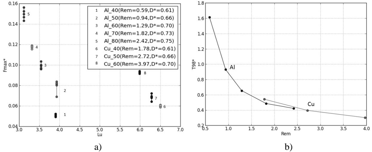
Figure 4: The maximum of the nondimensional Lorentz force as a function of the Lundquist number at different  $Re_m$  and  $D^*$  (a) and the nondimensional saturation time  $T_{98}^*$  for different  $Re_m$  (b).
