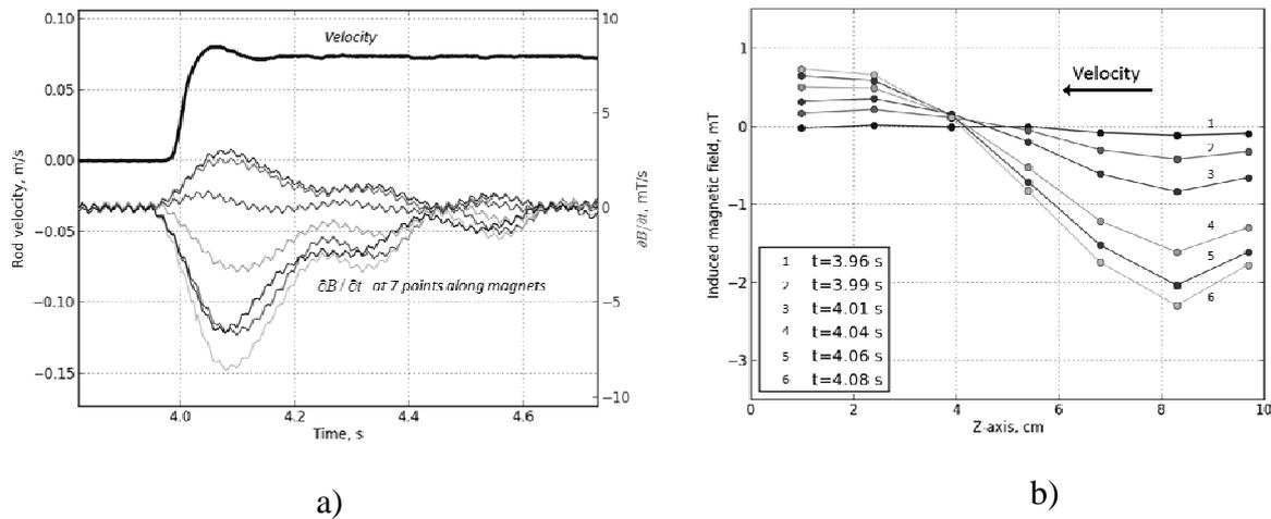
Figure 5: Time-derivative of the induced magnetic field (a) and its evolution in time (b).
