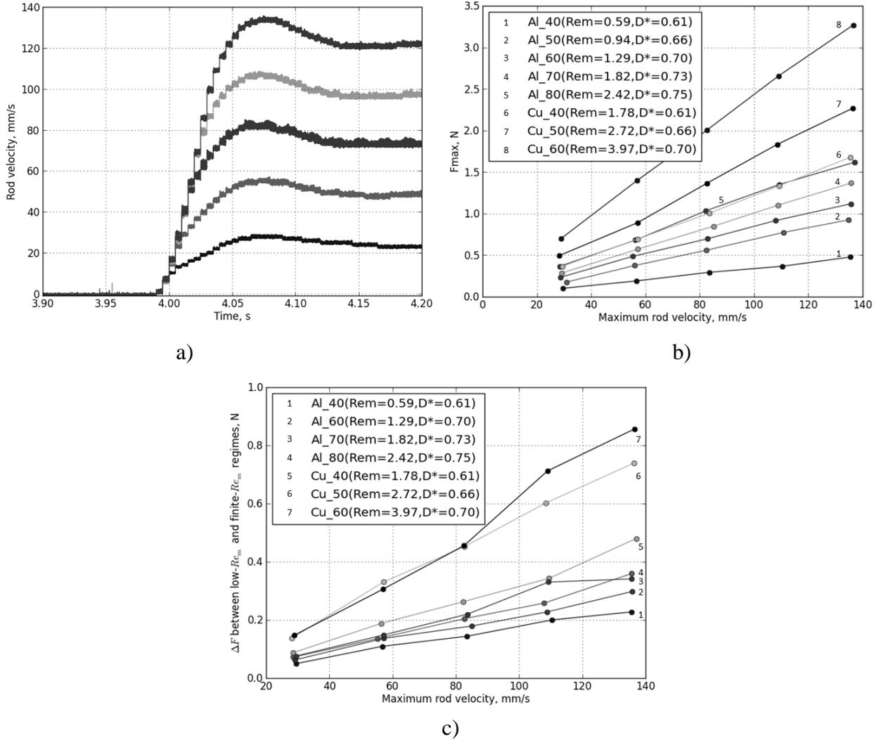
Figure 3: 5 different signals of the rod velocity (a), the maximum Lorentz force acting on the rod as a function of velocity at different  $Re_m$  and  $D^*$  (b), and the difference between low- $Re_m$  and finite- $Re_m$  cases (c).
