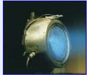
Ions are extracted from the plasma and accelerated out by a system of biased grids
