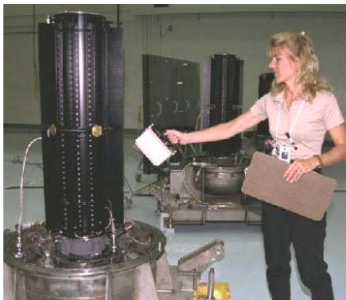
USA GPHS RTG (General Purpose Heat Source RTG). (1980s to 2000s.) 56kg. 295W e . 572 Si-Ge thermoelectric couples.
