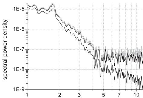
Fig. 4. Influence of tip spacing on turbulence spectra. Gray: backcalculated [10] from 1 mm; black: 1 and 5 mm.
