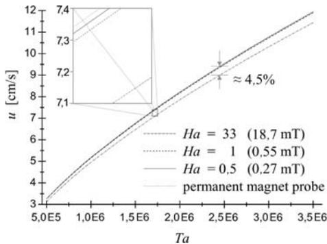
Fig. 2. Influence of the strength of the measuring magnetic field onto the swirling flow in an RMF.
