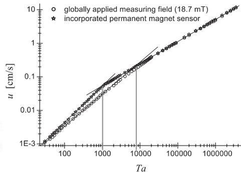
Fig. 3. Scaling of RMF-driven flow in the Stokes and laminar boundary layer regimes.
