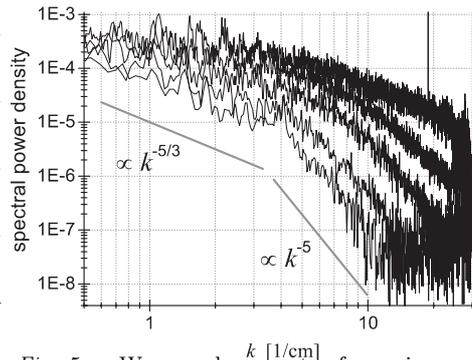
Fig. 5. Wavenumber spectra for various values of the Taylor number: 3.2E5, 5.6E5, 1.3E6, 2.9E6, and 7.9E6.
