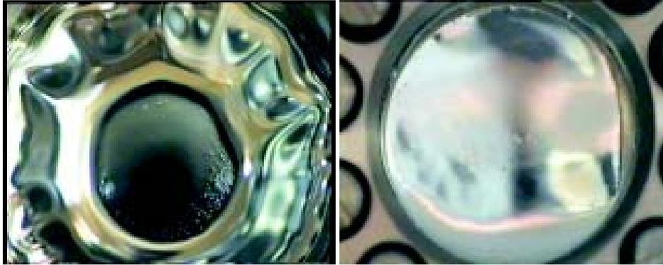
Fig. 5. The deformations of the Gallium melt region due to intense flow induced by thermo-electric current interaction with DC magnetic field: axially symmetrical video frame (left) and transverse one (right).
