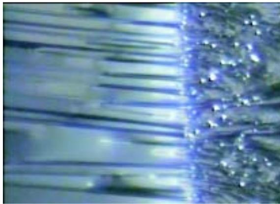
*Fig. 7.* Super fast crystallization of Gallium.
