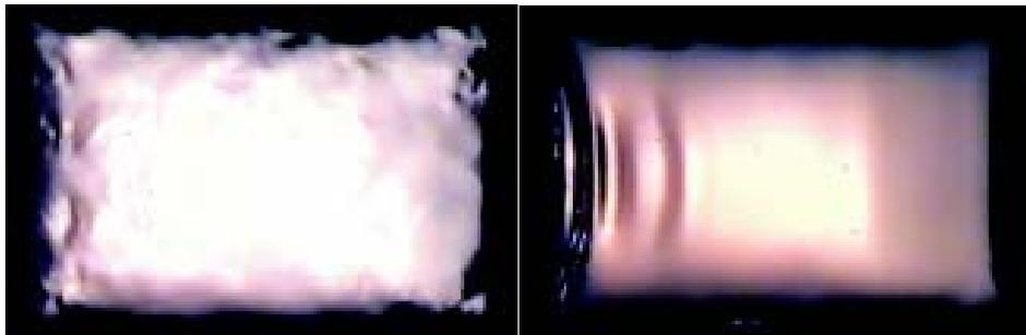
Fig. 2. AC field induced flow in liquid metal. The video frame on the right side illustrates the effect of the superimposed DC field normal to the longer side wall of the rectangular crucible.
