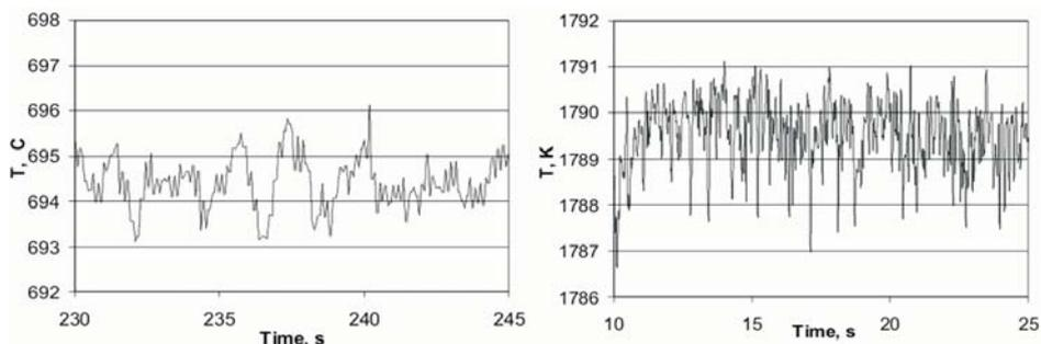
Fig. 4. Temperature oscillations on the axis measured in aluminium (left) and calculated for TiAl alloy (right).
