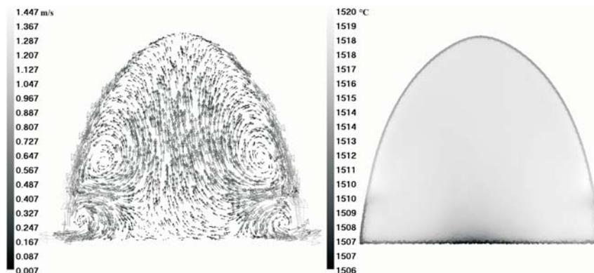
Fig. 3. Time averaged velocity and temperature distribution in TiAl alloy.
