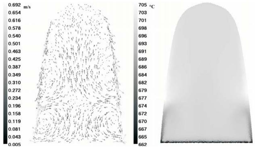
Fig. 2. Time averaged velocity and temperature distribution in Aluminium.
