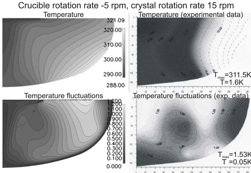
Fig. 2. The melt flow without any EM field influence. Numerically modeled (left) and measured (right) temperature and temperature fluctuation distributions (in K).
