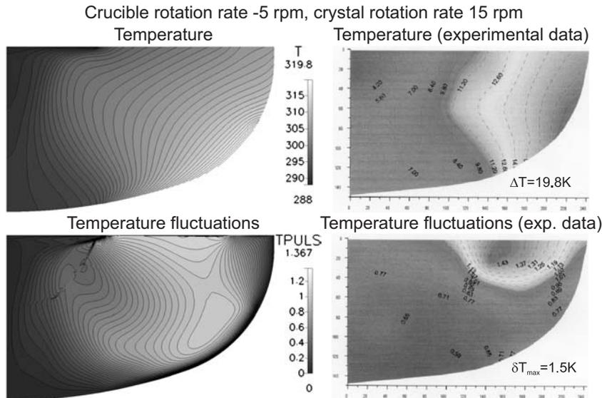
Fig. 4. The melt flow under the influence of the 70 – mT CUSP magnetic field. Numerically modeled (left) and measured (right) temperature and temperature fluctuation distributions.
