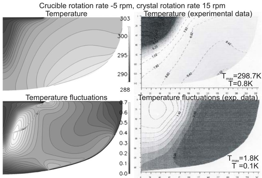
Fig. 3. The melt flow under the influence of the "down" TMF with  $60^\circ$  phase shift and 1667 Aw current strength. Numerically modeled (left) and measured (right) temperature and temperature fluctuation distributions.
