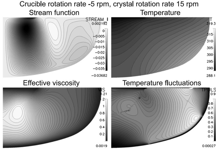
Fig. 5. The melt flow without any EM field influence. The results of numerical modeling with the modified low-Re-number  $k$ - $\varepsilon$  turbulence model. The meridional distributions of stream function ( $\text{m}^3/\text{s}$ ), temperature (K), effective viscosity ( $\text{Pa} \cdot \text{s}$ ), and temperature fluctuations (K).
