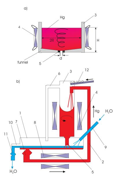
Fig. 1. (a) Formation of the funnel flow by the RMF; (b) schematic of the experimental setup. 20
