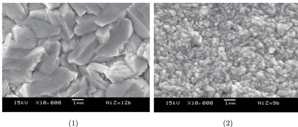
Fig. 3. SEM micrographies of Zn-Ni alloys deposited at  $-1.75$  V/SSE, pH = 3.5. Magnification  $\times 10\,000$  (white line represents  $1\ \mu\text{m}$ ) Photo 1:  $B = 0$ . Photo 2:  $B = 0.6$  T.
