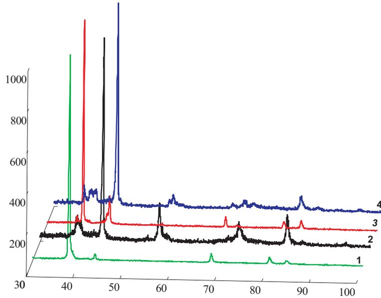
Fig. 4. XRD diagrams for Zn-Ni alloys. Electrodeposition has been realized at  $-1.75$  V/SSE. The intensities have been normalized. Curve 1 pH = 3.5;  $B = 0$ . Curve 2 pH = 3.5;  $B = 0.6$  T. Curve 3 pH = 2.5;  $B = 0$ . Curve 4 pH = 2.5;  $B = 0.9$  T.
