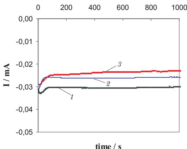
Fig. 2. Chronoamperometric curves for electrodeposition of Zn-Ni. Applied potential =  $-1.75$  V/SSE. Line 1 pH = 3.5;  $B = 0.6$  T; line 2 pH = 3.5;  $B = 0$ ; line 3 pH = 2.5;  $B = 0$ .
