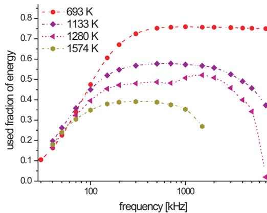
Fig. 4. Optimization of ICF frequency by glass-melting – the average temperature of the load is fixed.
