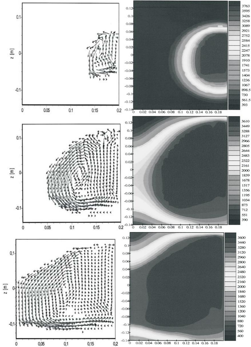
Fig. 3. Distributions of velocity and temperature in ICF by  $ZrSiO_4$  melting at different time moments:  $t = 29, 5$  min;  $55, 3$  min;  $59, 5$  min.
