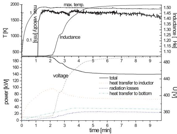
Fig. 2. Changes of power parameters, voltage, maximal temperature, velocity and inductance by inductive heating with 5100 A of 7.9 kg of TiAl melt.
