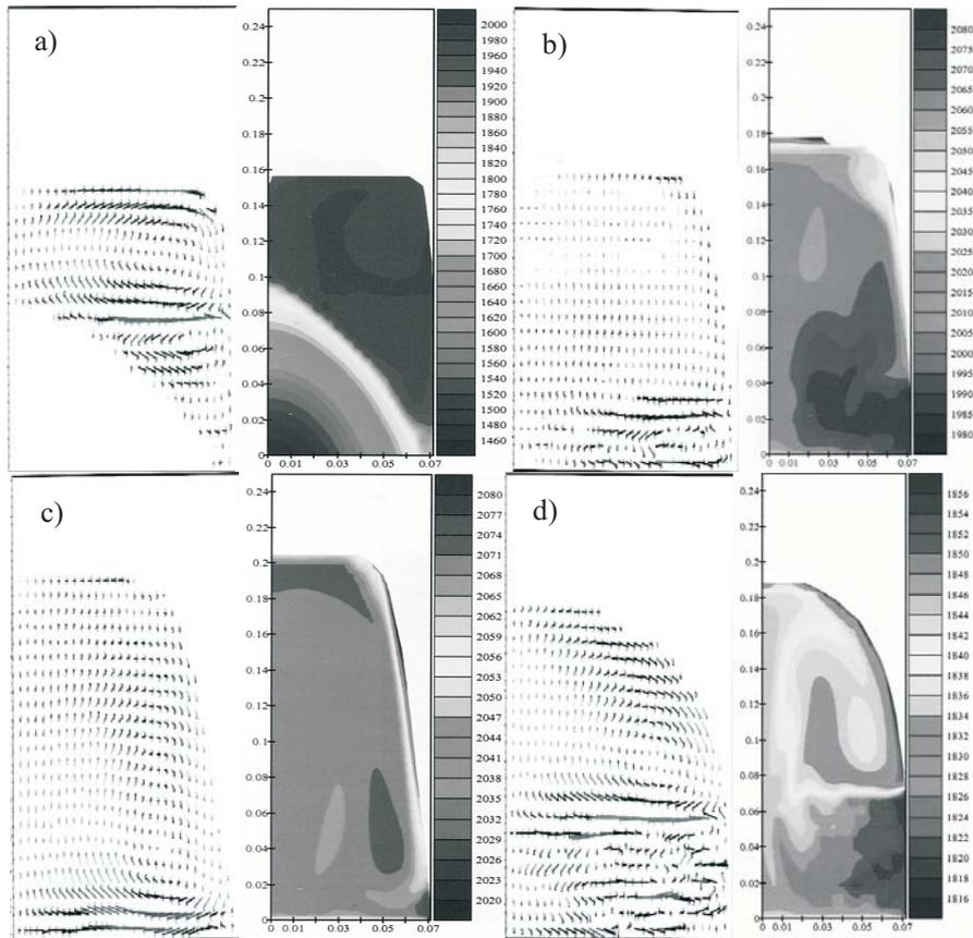
Fig. 1. Distributions of velocity and temperature in the load (TiAl) by IFCC melting at different time moments: a)  $t = 5,72$  min ( $I = 6500$  A); b)  $6,57$  min ( $I = 6500$  A); c)  $7,05$  min ( $I = 6500$  A); d)  $8,6$  min ( $I = 4000$  A).
