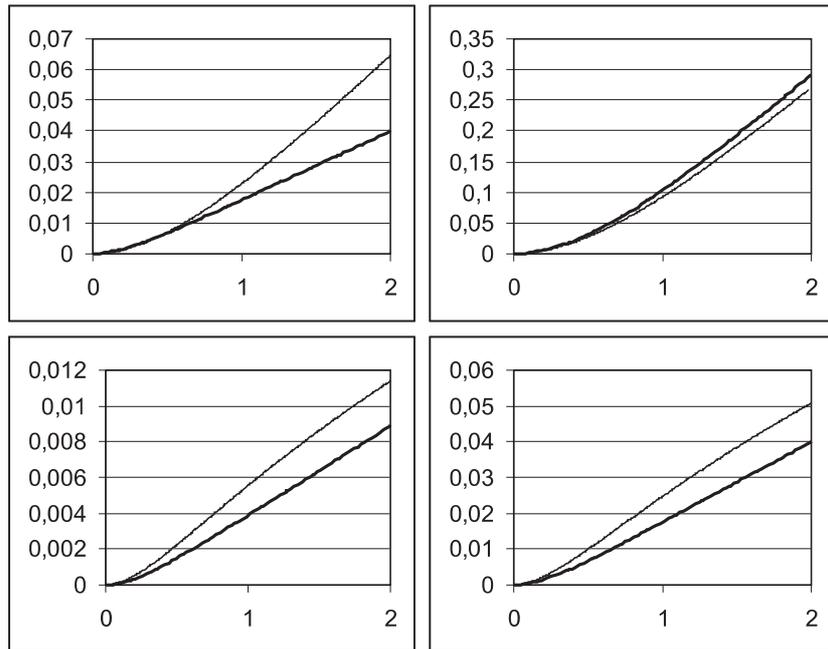
Fig. 3. Configuration of a flexible magnetic rod. Tight line – non-linear model, bold line – linear model. Left top –  $C_m = 1$ ,  $F_a = 0.1$ ; right top –  $C_m = 1$ ,  $F_a = 0.45$ ; left bottom –  $C_m = 10$ ,  $F_a = 0.1$ ; right bottom –  $C_m = 10$ ,  $F_a = 0.45$ .
