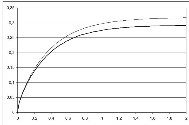
Fig. 1. Displacement of the end of the rod.  $C_m = 1$ ,  $F_a = 0.45$ . Tight line – non-linear model, bold line – linear model.
