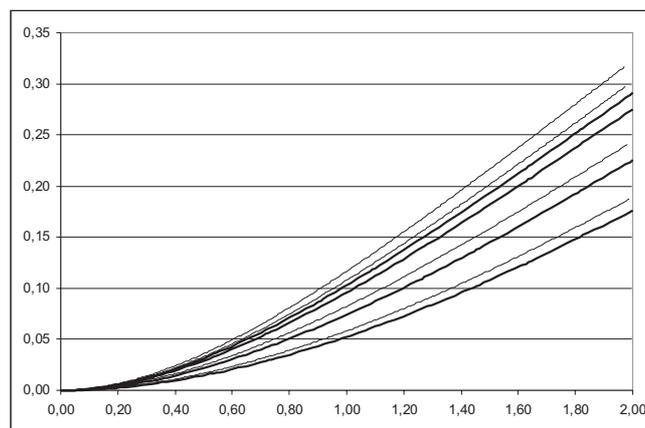
Fig. 2. Configuration of a rod  $C_m = 1$ ,  $F_a = 0.45$ . From lower to upper  $\tau = 0.3, 0.5, 1, 2$ . Tight line – non-linear model, bold line – linear model.
