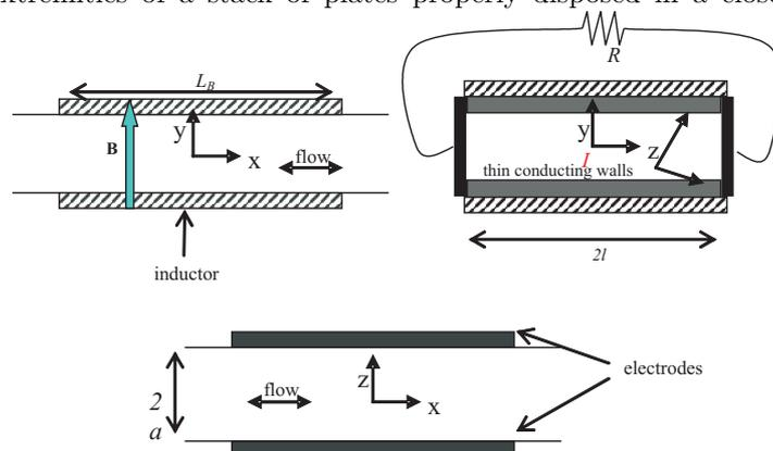
*Fig. 1.* Views of the MHD channel, the electromagnetic inductor creates a vertical magnetic field; the resulting current lines are collected by the electrodes.
