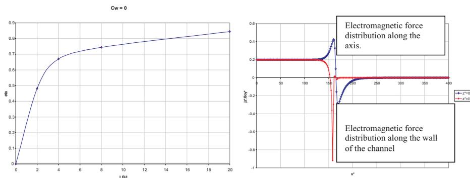
Fig. 3. Maximum efficiency versus the aspect ratio for  $\delta^* = 2.5$ ,  $C_w = 0$ . The more the aspect ratio, the more the MHD channel is near an infinite channel, then the efficiency tends toward the maximum value of an infinite channel.
