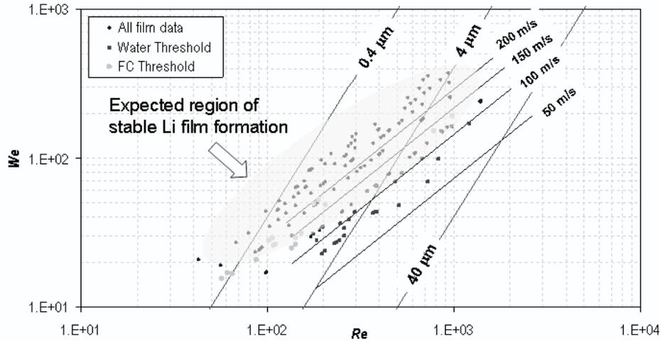
Fig. 1. Film stability diagram using FC-3283 and water.
