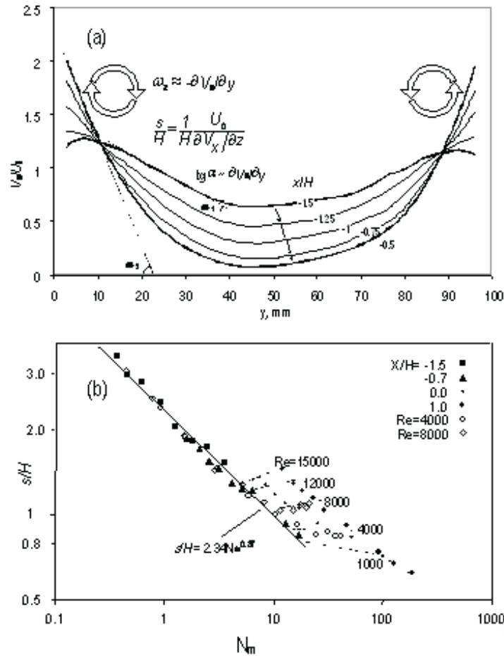
Fig. 1. Transformation of mean velocity profile. (a) Stream wise component of velocity  $V_x$  at the different distances  $x/H$  with respect to the magnet center,  $Re = 4000$ ,  $U_0 = 8$  cm/s – mean flow rate velocity,  $\omega_z$  – vertical component of vorticity,  $s/H$  – dimensionless thickness of the side boundary layer,  $H = 20$  mm – height of the flow. (b) Dependence of the side boundary layer thickness  $s/H$  on the modified Stuart number  $N_m$ .
