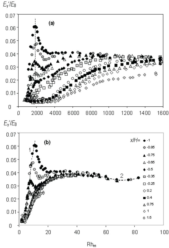
Fig. 2. Intensity of electric potential fluctuations ( $E'_y/E_0$  in the region of applied magnetic field in the central part of the channel ( $y = 0$ ) versus the (a) Reynolds number and (b) the modified  $Rh_m$  number.  $x/H$  – dimensionless distance from the center of the magnet. The negative and positive values correspond to the space before and past the magnet respectively.  $E_0$  – strength of electric potential corresponding to the mean flow rate velocity.
