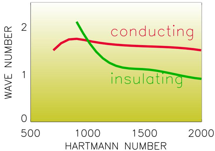
Fig. 4. Wave numbers, for which the Reynolds number is minimum for conducting walls and insulating walls. ( $Pm = 10^{-5}$ , Rüdiger & Shalybkov 2002).
