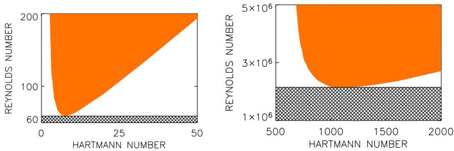
Fig. 2. Marginal stability lines for axisymmetric modes in containers with a rotating outer cylinder of conducting material for  $Pm = 1$  (left) and  $Pm = 10^{-5}$  (right).  $\hat{\eta} = 0.5, \hat{\mu} = 0.33$ . The instability domain is grey-colored and fluids in the cross-hatched area are always stable.
