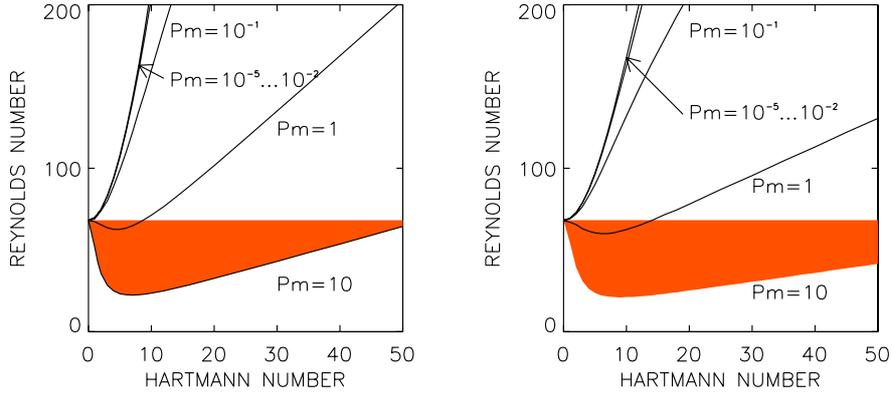
Fig. 1. Bifurcation diagram for axisymmetric modes with a resting outer cylinder of conducting material (left) and vacuum (right). Shaded areas denote subcritical excitation by the axial magnetic field.  $\hat{\eta} = 0.5$ . From Rüdiger, Schultz & Shalybkov (2003).
