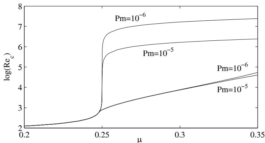
Fig. 5. Critical Reynolds numbers in containers ( $\hat{\eta} = 0.5$ ) with a purely axial magnetic field (upper curves) and with an extra toroidal field (lower curves) for  $\text{Pm} = 10^{-5}$  (sodium) and  $\text{Pm} = 10^{-6}$  (gallium). The cylinders are insulators. The Prandtl number dependence of the lower curves is extremely weak and the Reynolds numbers are strongly reduced (Hollerbach & Rüdiger 2005).
