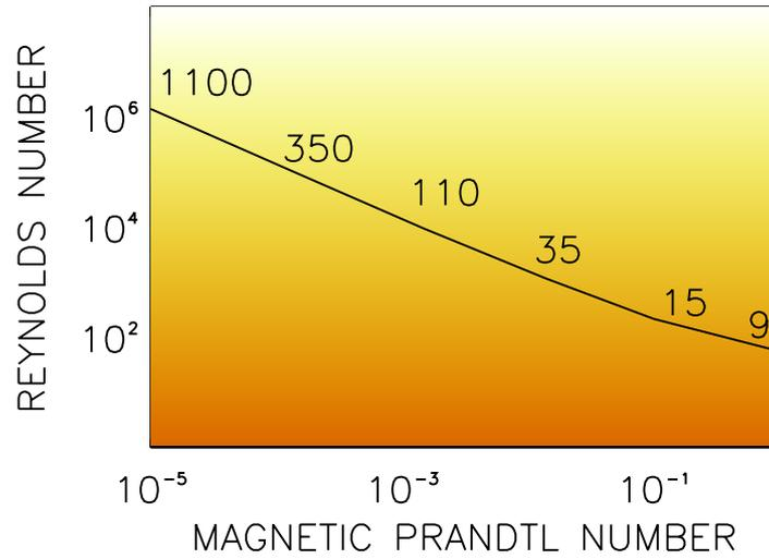
Fig. 3. The critical Reynolds numbers vs. the magnetic Prandtl numbers marked with those Hartmann numbers where, the Reynolds number is minimum.  $\hat{\eta} = 0.5$ ,  $\hat{\mu} = 0.33$ .
